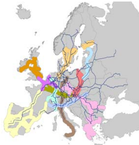
Figure 4.1: Rail-based shipment routes (blue lines) coincide with the TEN-T intermodal priority axes (colours). REORIENT shipper survey
