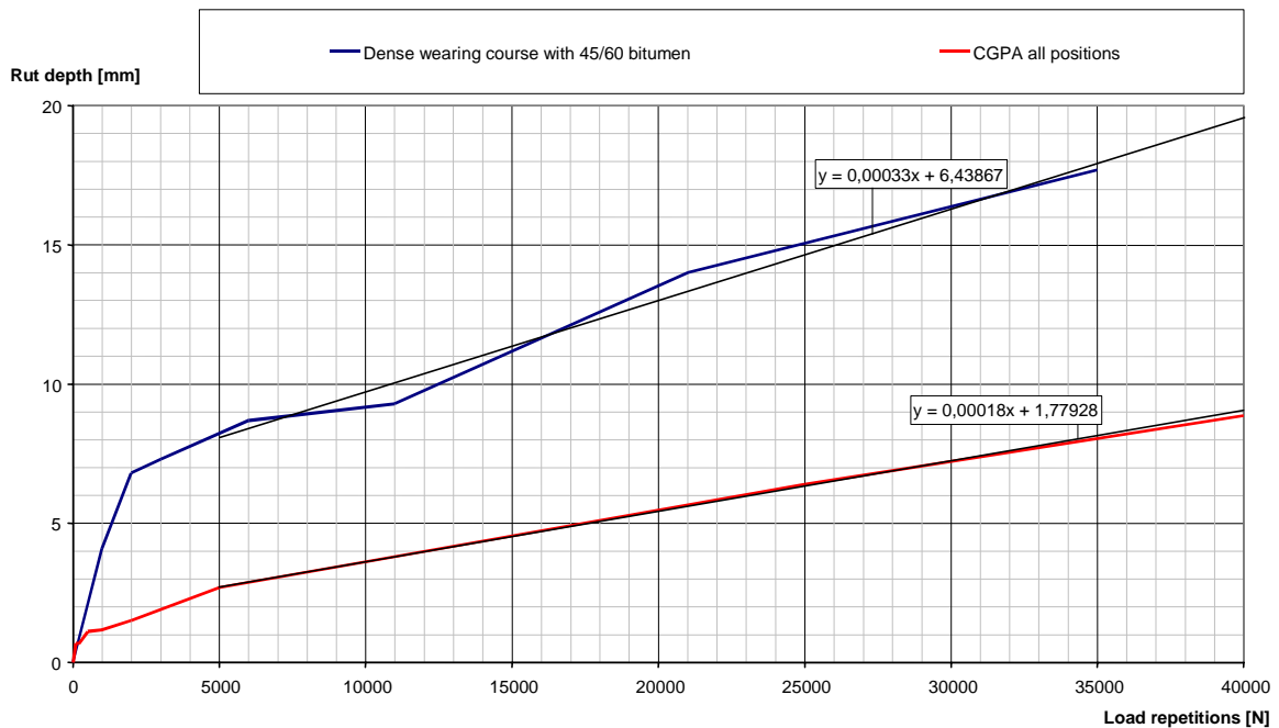
Figure 6.4 - Comparison of rutting behaviour of cement grouted porous asphalt wearing course (CGPA) with results from the conventional dense asphalt wearing course (DAC) with 45/60 bitumen - DWW
