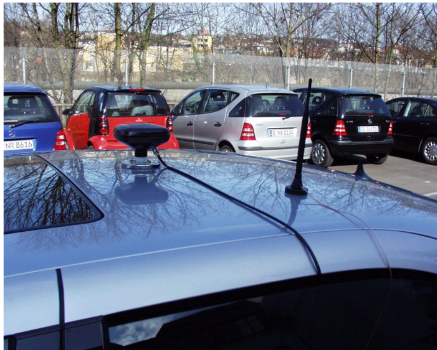
Figure 18 – GPS-antenna (left) and WLAN-antenna (right)
