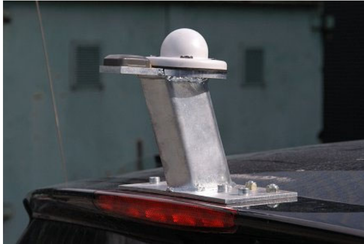
Figure 23 – WLAN antenna on roof of Smart
