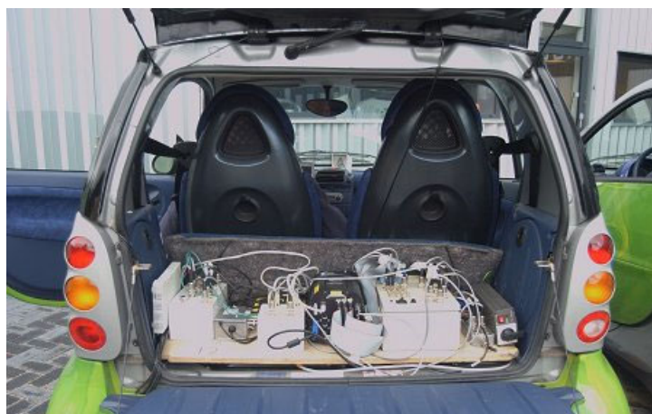
Figure 25 – Integration of equipment in trunk of vehicle
