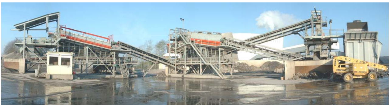
Figure 2-34 (below): Photos of an outdoor installation for processing reclaimed asphalt concrete
