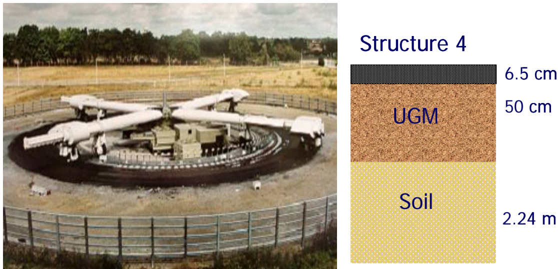
Figure 2-18: View of the LCPC accelerated pavement testing facility and pavement structure used for modelling
