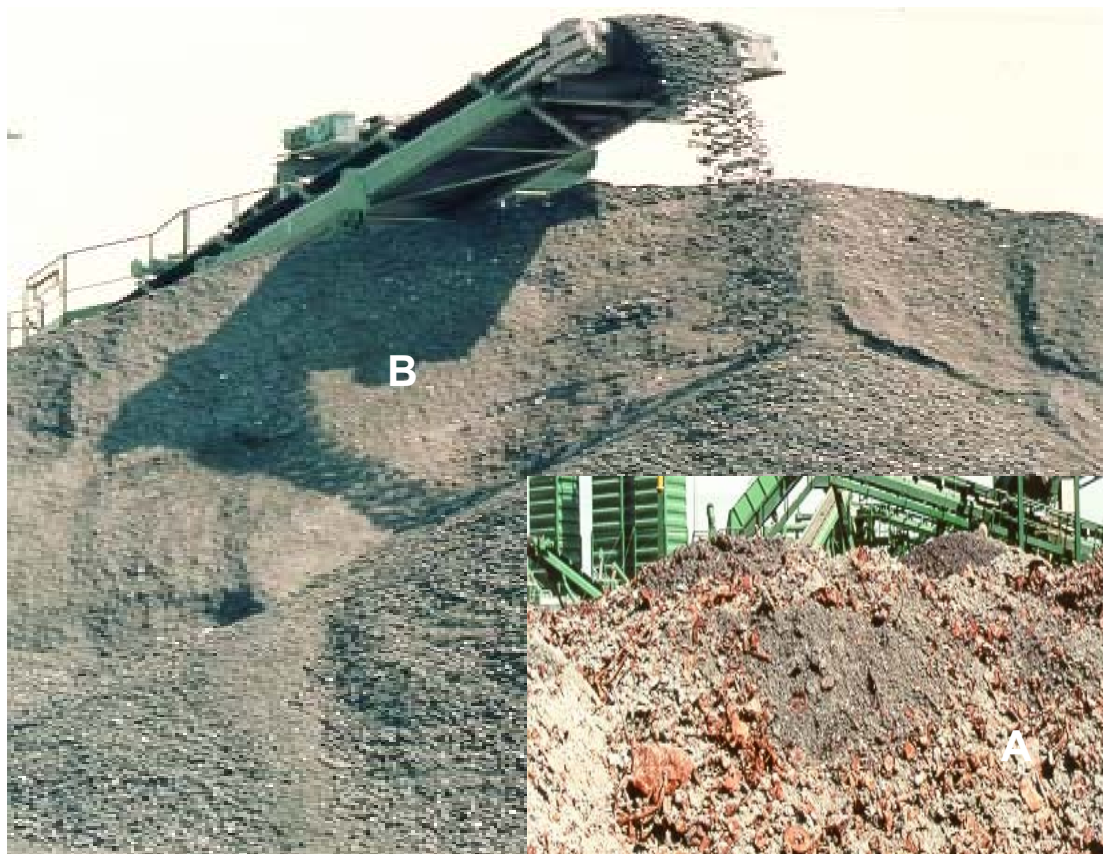
Figure 2-33: A : Fresh bottom ash – B : Processed bottom ash
