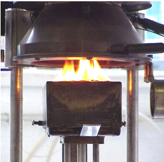
Cone Calorimeter ISO 5660-1 test equipment
