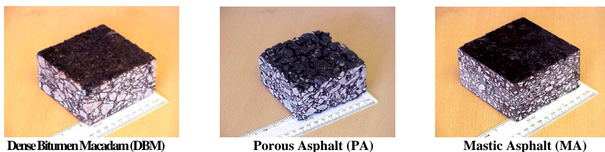
Figure 2-6: Pavement materials selected for testing for their reaction to fire.
