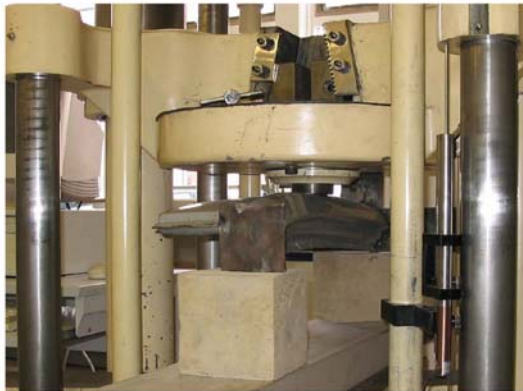
Figure 39: Pre test side roof rail
