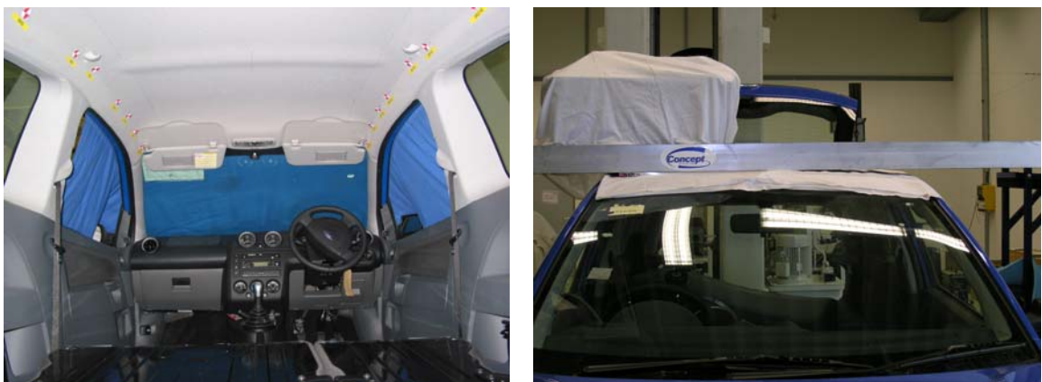
Figure 26: FMH-testing points: Left: Normal test points; Right: Weight (300kg) on roof of the car
