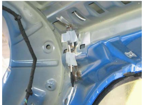
Figure 24: Left: Accelerometer 'car3' (Top of B-Post cant rail); Right: Accelerometer 'car4' (Rear of cant rail by tailgate)
