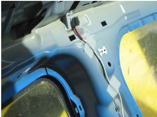
Figure 24: Left: Accelerometer 'car3' (Top of B-Post cant rail); Right: Accelerometer 'car4' (Rear of cant rail by tailgate)
