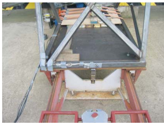
Figure 25: Left: Accelerometer 'car5' (Sill by B-Post); Right: Accelerometers 'sled1' and 'sled2' (Rear of sled)
