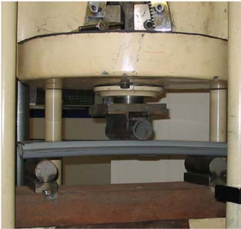
Figure 41: Pre test header rail
