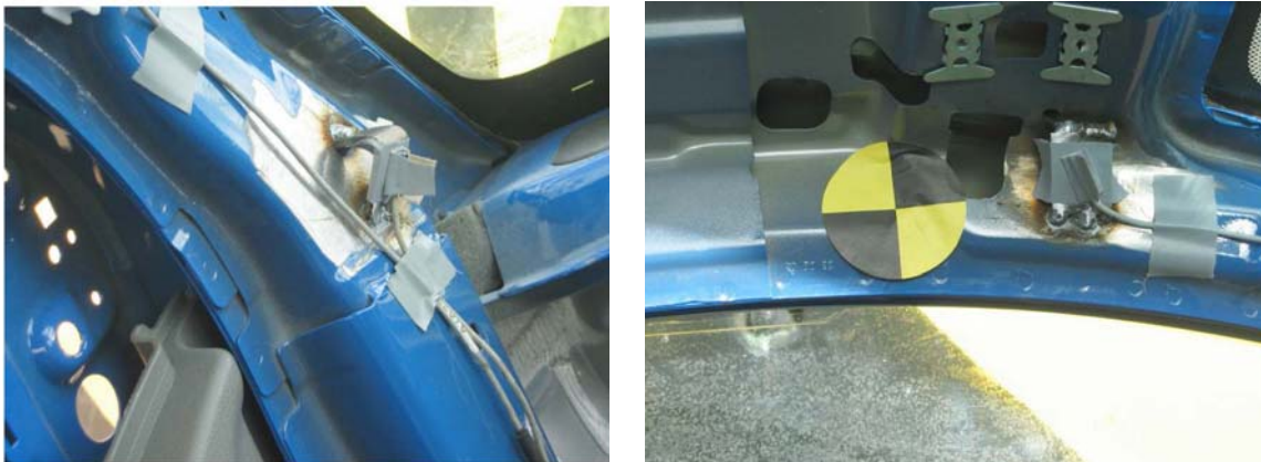
Figure 23: Left: Accelerometer 'car1' (LH A-Post by base of windscreen); Right: Accelerometer 'car2' (Top of A-Post by header rail)
