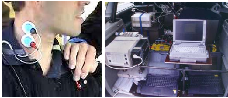
Figure 4: Electrodes measuring activity of the right m. sternocleidomastoideus (left), technical equipment in the car boot (right)
