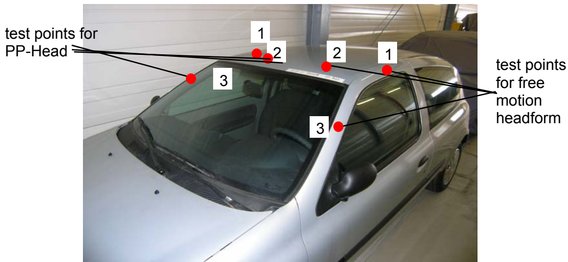
Figure 9: Test points for pedestrian protection head and free motion headform
