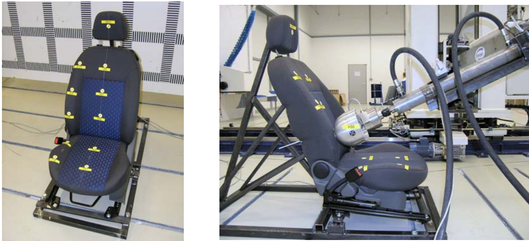
Figure 45: Left: Test points on Seat; Right: Test Setup
