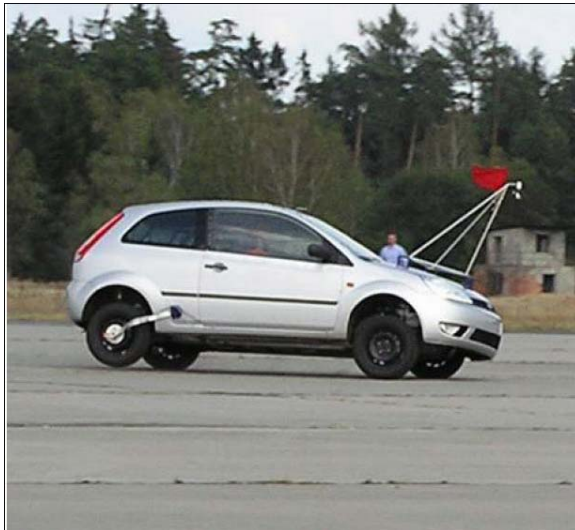
Figure 4: Vehicle at T = 4.2 s, stationary after steering 33 degrees to the right
