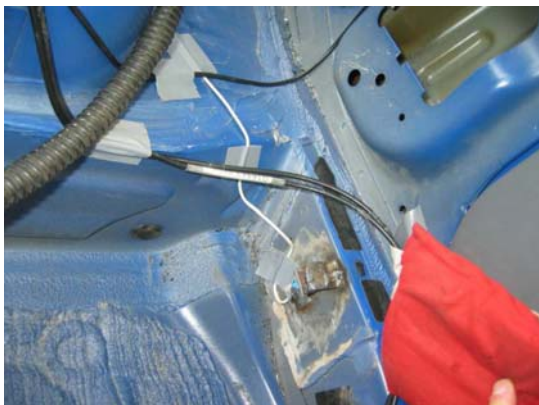
Figure 25: Left: Accelerometer 'car5' (Sill by B-Post); Right: Accelerometers 'sled1' and 'sled2' (Rear of sled)
