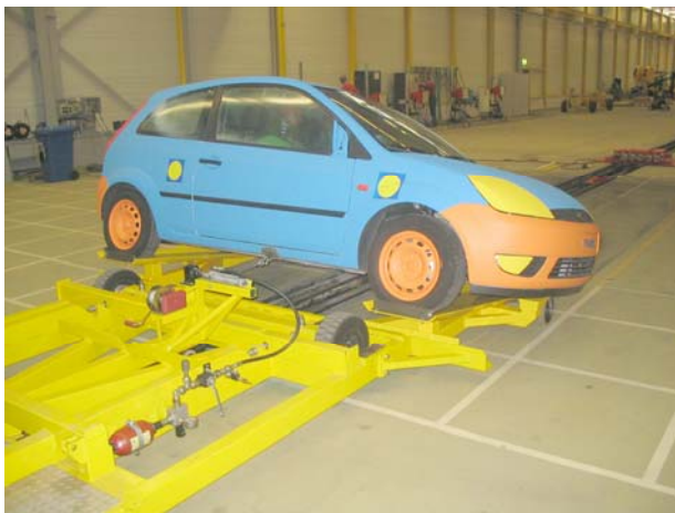
Figure – TNO Rollover Test Setup
