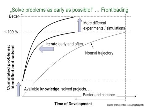
Fig. 4.2.2: The frontloading concept of Up-Front Simulation
