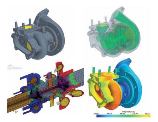
*Fig.4.5.6.3: Turbocharger compressor and turbine complete assembly (top right), continuous multi-domain meshing incorporating fluid-side surface mesh extrusions (bottom left), flow and thermal solutions (right)*
