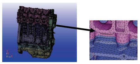
Fig. 4.5.4.1: Example of automatic assembly meshing (courtesy of Techno-Star Europe GmbH)
