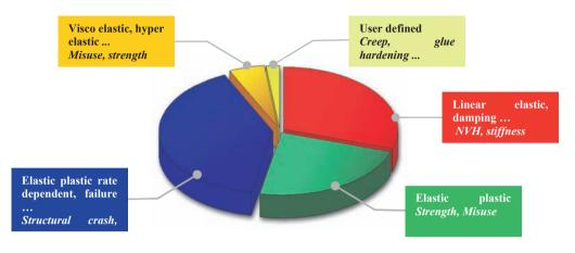
Fig.4.3.3.1: Distribution of material models in current use (courtesy of P&Z)
