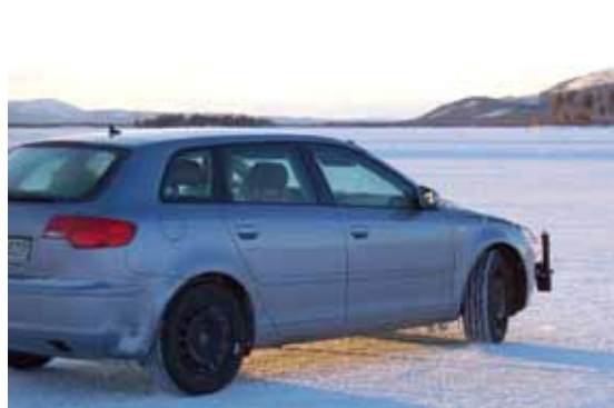
NIRA car with speed sensor mounted at the front
