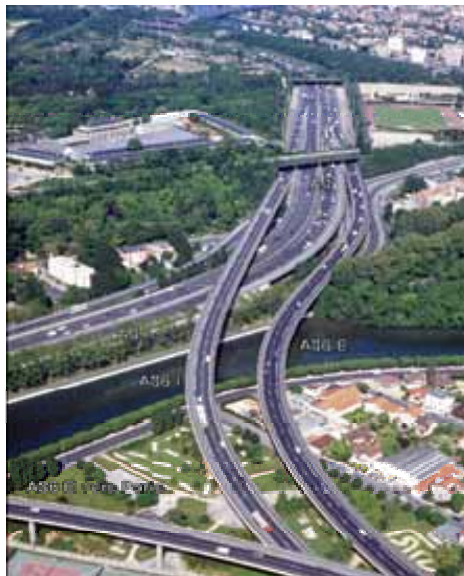
Figure 26: A4-A86 Weaving section in France
