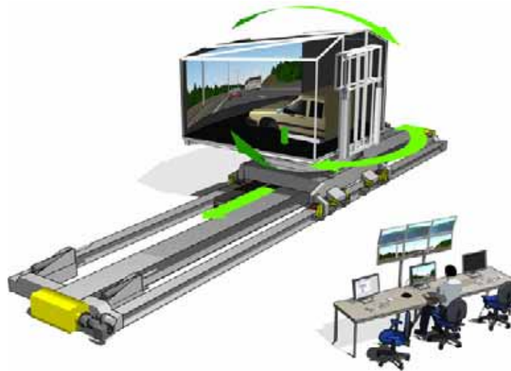
Figure 20: The VTI Driving Simulator III. The arrows indicate possible movements.
