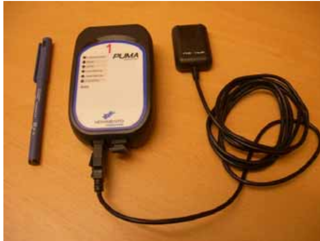
Figure 3: PUMA, the CAN bus logger used in Sweden
