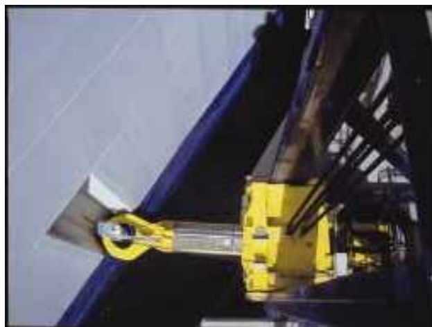
Figure 4.12. Automoorings unit in activated position, seen from above
