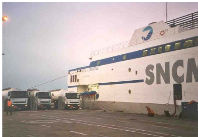
Figure 3.12 Tank lorries providing fuel to an HSC in the Port of Nice
