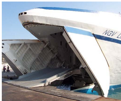
Figure 3.4 Ramp built on the NGV Liamone
