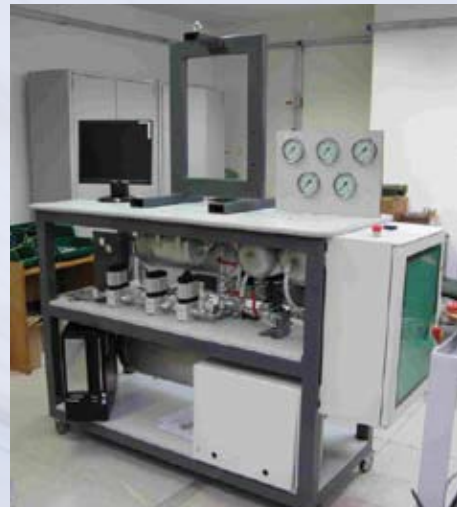
Testbench to assess functionalities and fault tolerance of the Brake Control Unit.
