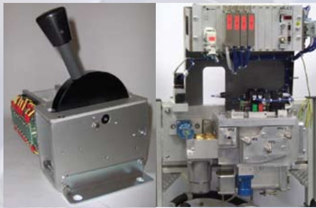
Components of the brake control unit: The brake handle (left) and the brake panel for the direct and the indirect brake architecture (right)
