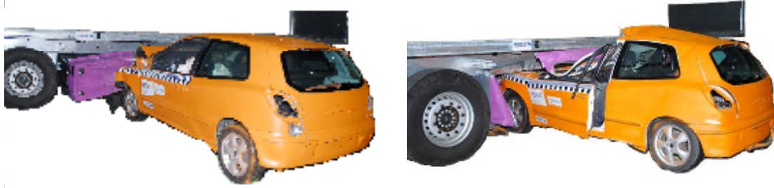
Figure 77: Full scale testing of crashworthy pallet box, versus full scale testing of conventional pallet box
