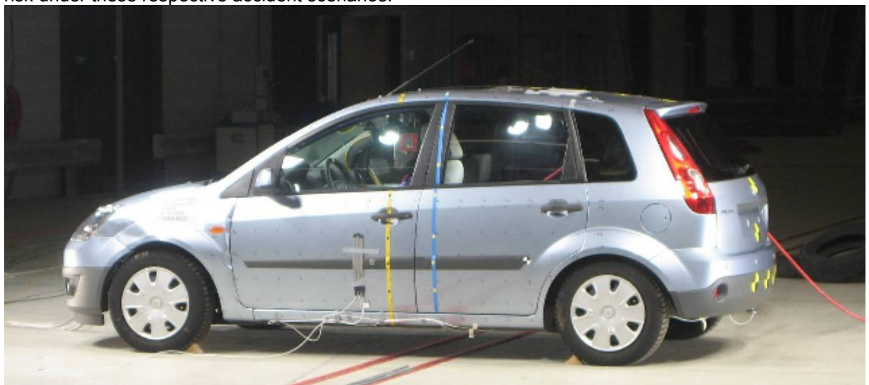
Figure 41: WorldSID revision 1 prototype first time in full scale car crash
