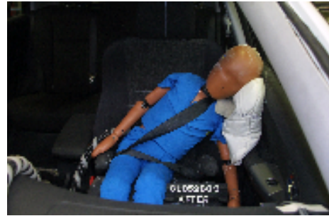
Figure 69: OOP test with CRS
