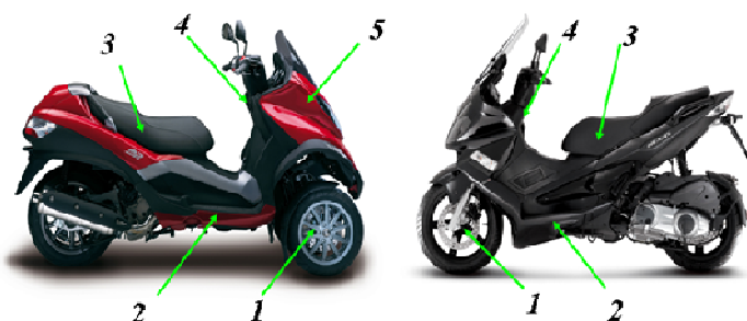
Figure 60: Piaggio MP3 250 and Gilera Nexus 500 showing sensor positions
