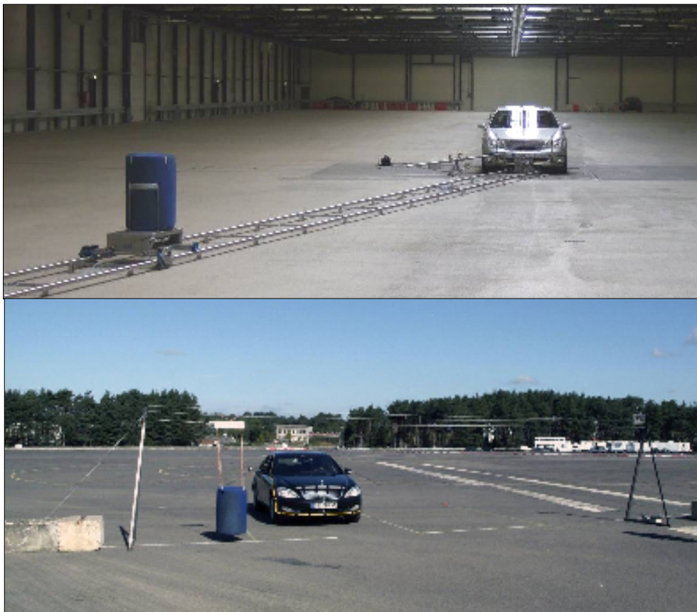
Figure 47: upper: moving platform with test object; in-door-testing. Lower: rope-way with foam block as test object
