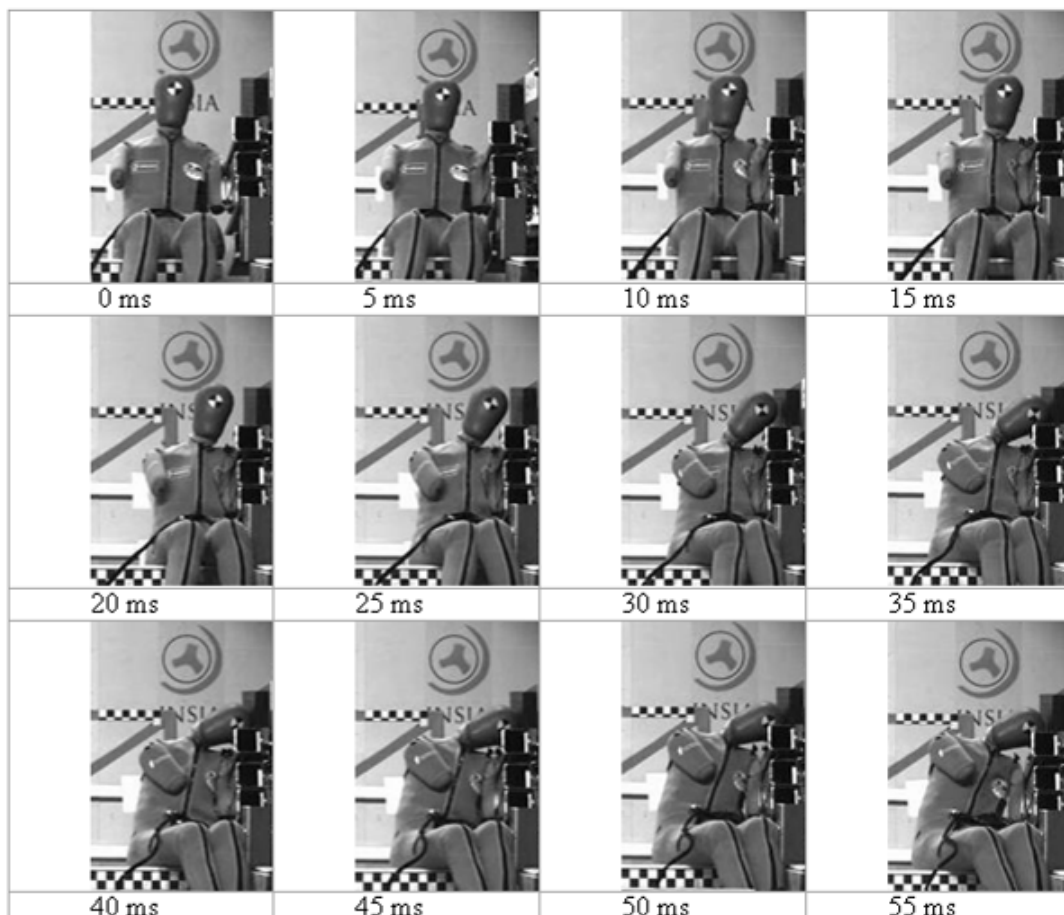
Figure 40: WorldSID small female in a sled test sequence of high speed video images
