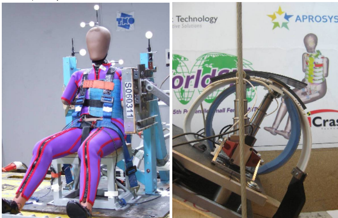
Figure 39: left: WorldSID small female dummy in testing, right: Oblique isolated rib unit test on drop tower, with new 2D-IR-tracc deflection sensors
