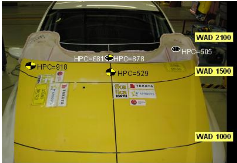
Figure 72: Head impact results, all acceptable
