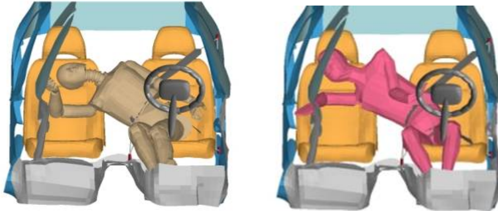
Figure 34: Dummy model (left) and active human model (right) in non-struck side lateral impact. The human model's head impacts the passenger's window, the dummy model does not
