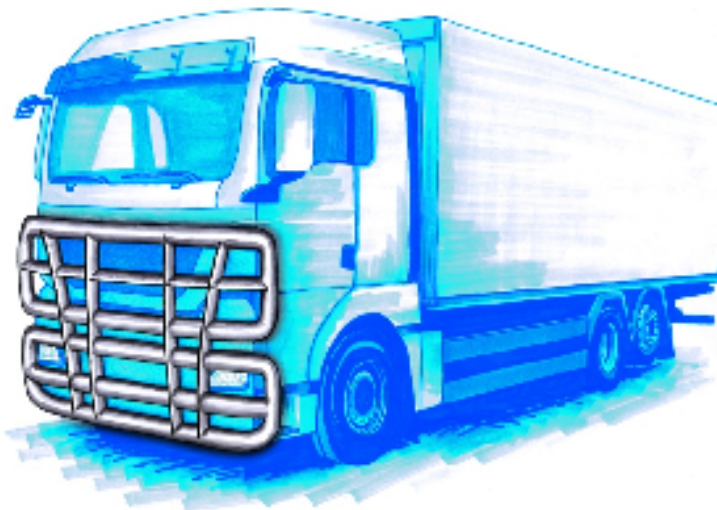
Figure 76: SafetyBar as styling feature and vulnerable road user protection device
