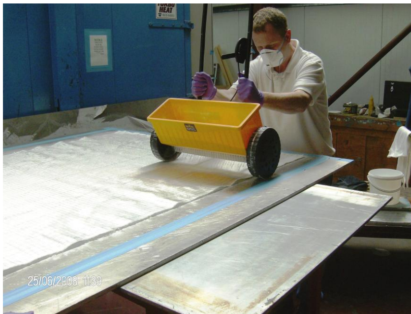
Figure 6: Sprinkling CBT®160 onto dry reinforcement
