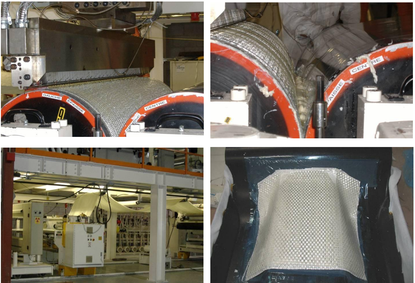
Figure 10: Davis-Standard modified extrusion coating process to make pre-preg with excellent drape
