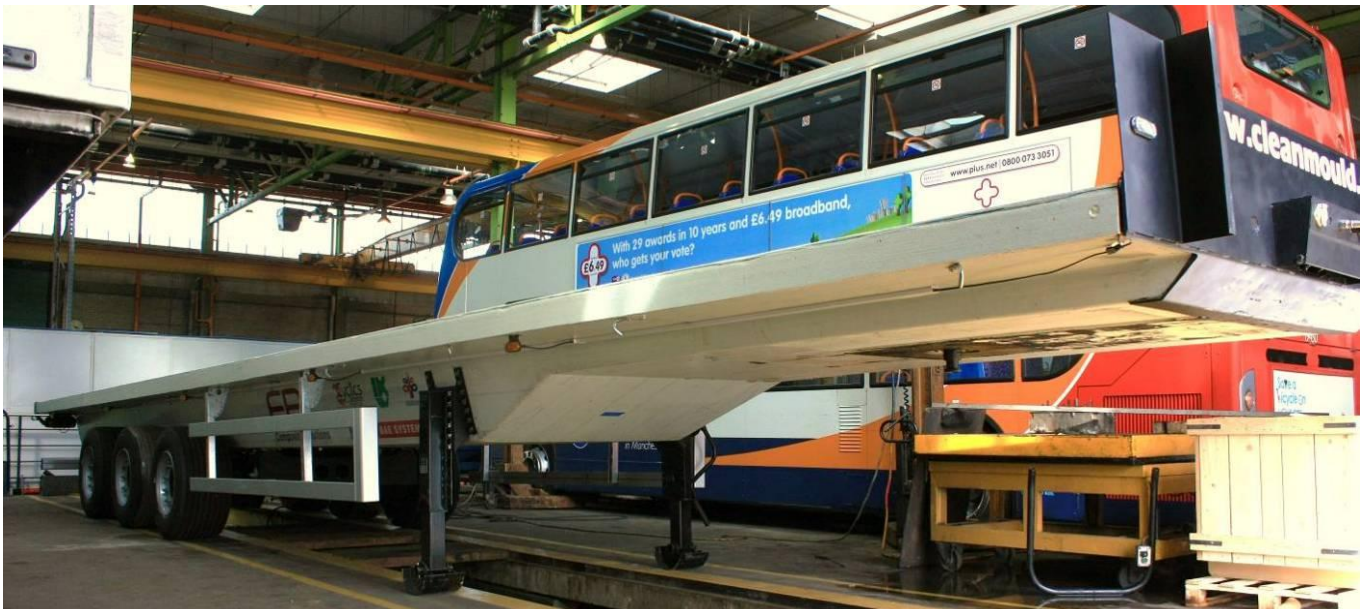
Figure 34 Trailer at Test House Undergoing Initial Static Load Tests
