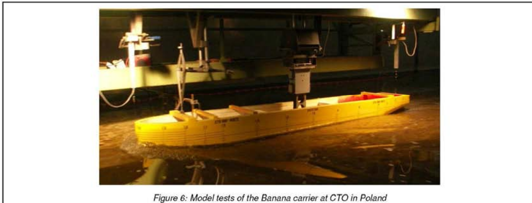
Figure 6: Model tests of the Banana carrier at CTO in Poland
