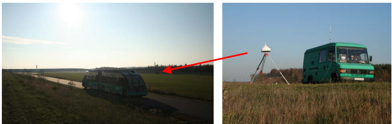
Figure 31: Test of the GPS (DGPS) based energy management strategy on the test side
