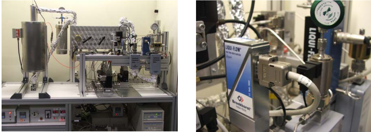
Figure 20: Dedicated setup for studies on LPG reforming
