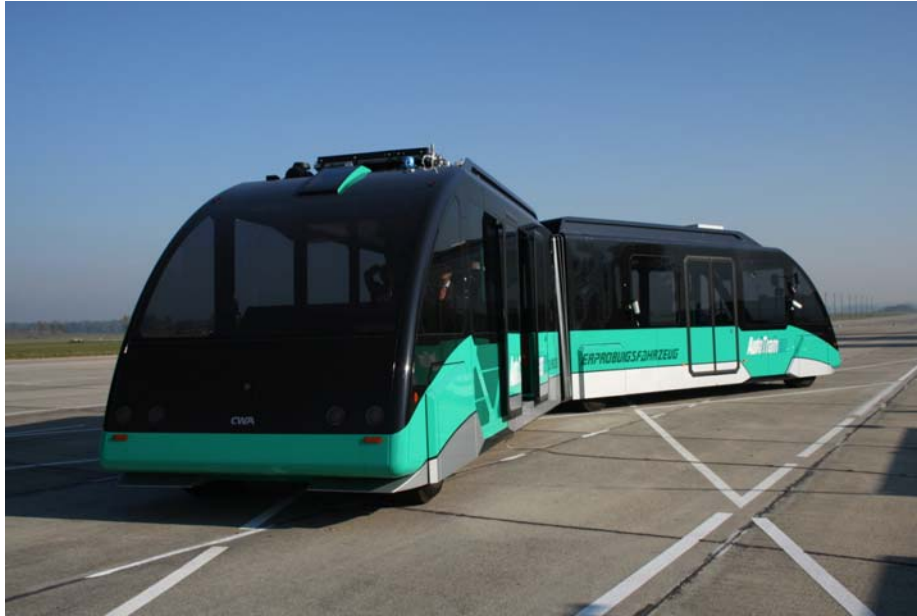
Figure 7: AutoTram test vehicle for PEFC cluster
