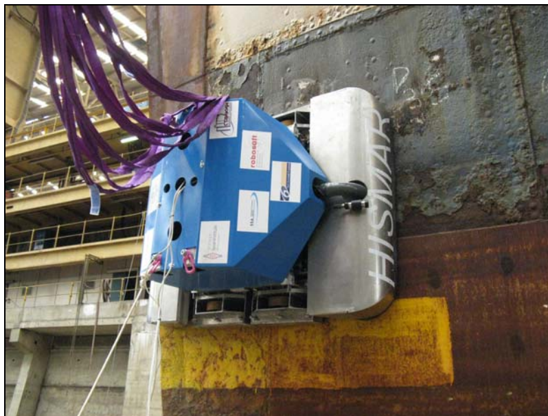
Figure 5: The completed Prototype HISMAR robot attached to a ship during field trials
