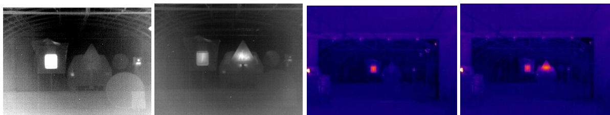
Figure C.3.13: Infrared images: MWIR in grey levels (non active panel on left and active on right) LWIR in pseudo colour levels (non active panel on left and active on right) – V = 22 m
