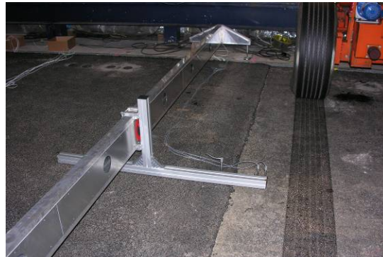
Figure C.1.3: Specific deflection beam used in the ALT facility
