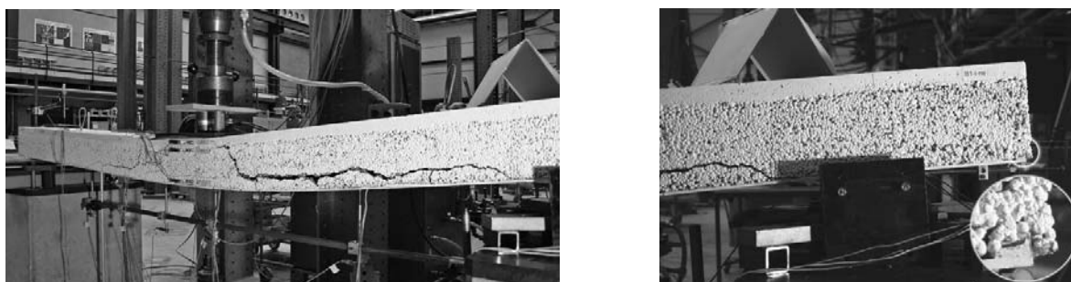
Figure 5 Failure pattern of unbonded SLWAC beam 1300-1 and slippage of LC from FRP sheet
