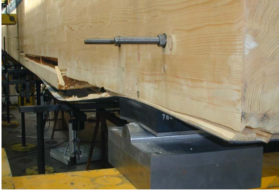
Figure 22 : Final failure, tensile cracking and propagation within timber, P1 beam.
