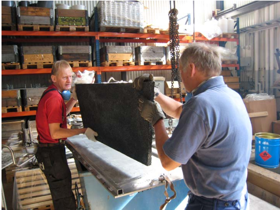
Figure C.5.4: Production of test material. Releasing the finished material from the mould.
