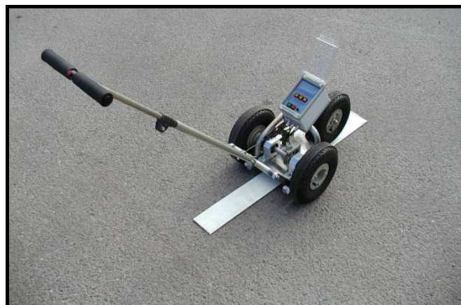
Figure C.5.7: The Portable Friction Tester used for measuring the wet friction coefficient at walking speed on the poroelastic surfaces. In the figure the PFT is placed with the measuring wheel on a road marking.
