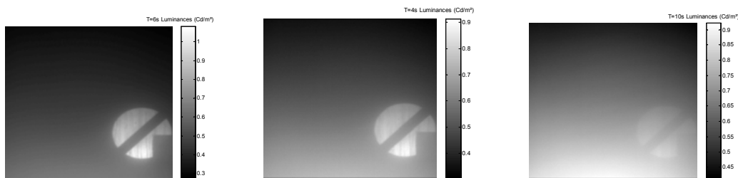
Figure C.3.12: Images acquired in the visible spectrum with the Videophotometer with car Headlights and for different meteorological visibilities: left V= 20 m – middle V = 15 m – right V= 12 m
