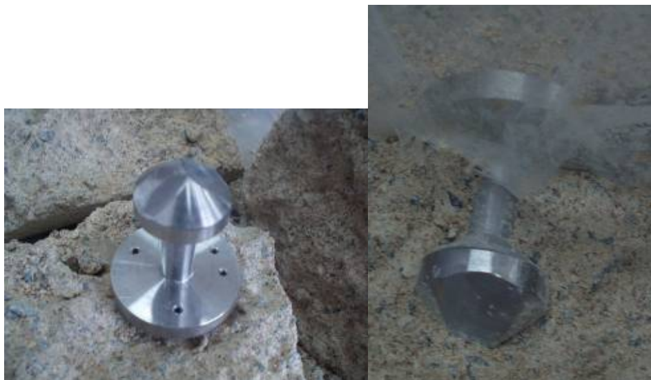
Figure C.2.7: Selected version of insert, with flat plates on the conic part, is well anchored
