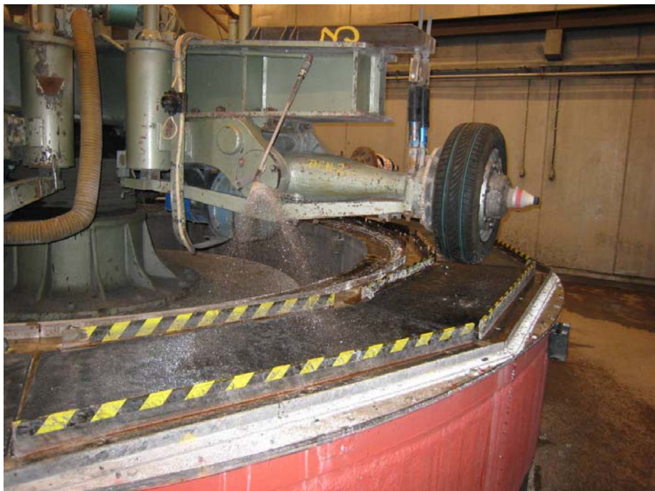
Figure C.5.6: The surfaces were sprinkled with water @ 6-8 L/minute during the accelerated traffic polishing tests.
