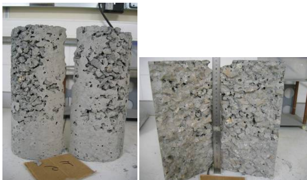
Figure C.2.3: Pictures of the F1 mix after curing. Segregation is due to the gap graded skeleton. Cracks are visible as well as brown scaling due to quicklime hydration in slag particles
