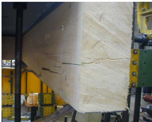
Figure 21 : Tensile cracking and propagation within timber, P2 beam (after post-mortem sawing)
