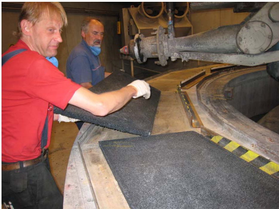
Figure C.5.5: Production of test material. Mounting the material in the PVM.
