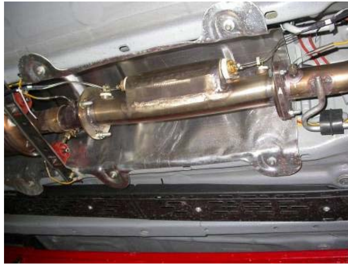
Figure 5.2.1 Photograph of The UV Optical Fibre Gas Sensors Mounted Underneath the Vehicle.
