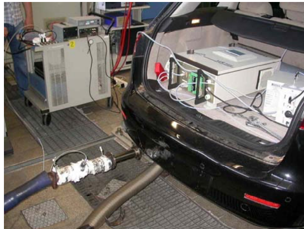
Figure 5.1.3. The Fiat Croma Demonstrator Undergoing Testing at the Roller Test Bench Facility
