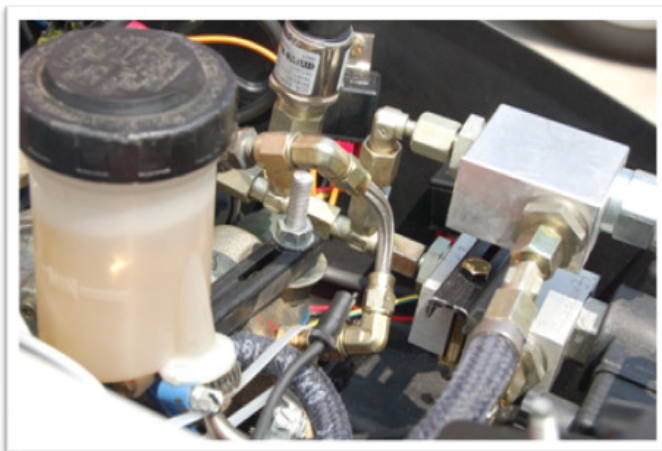
Figure 10: The installed Active Braking system
