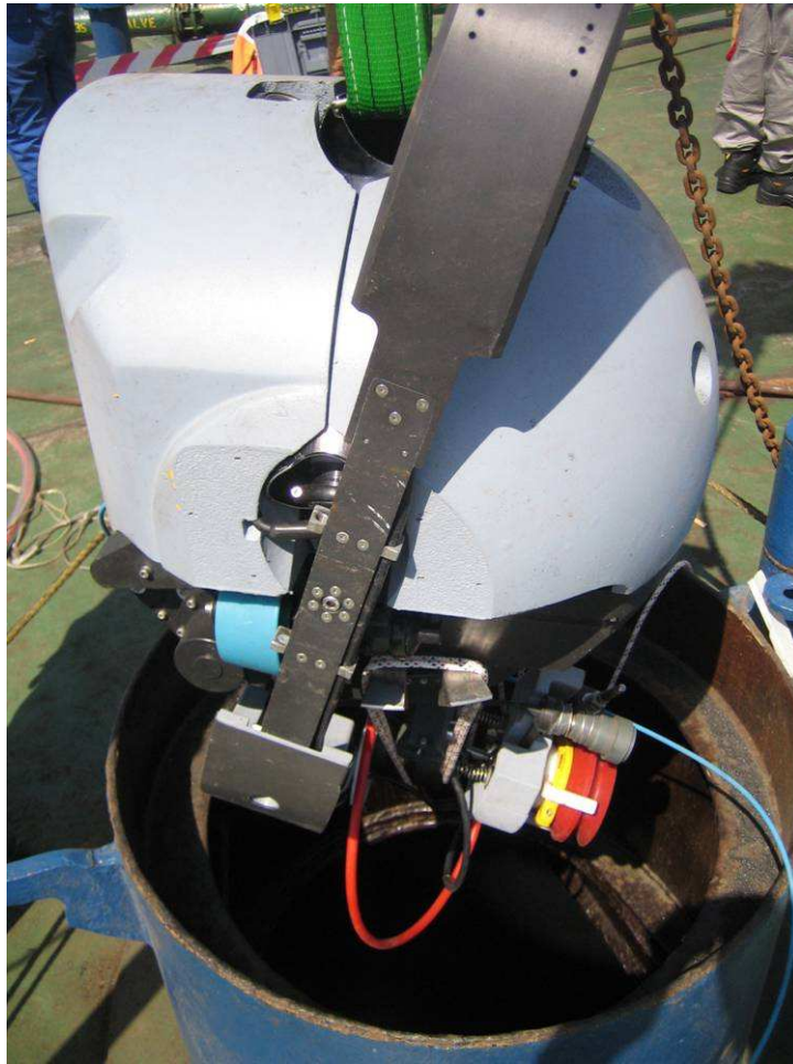
Figure 4 Inserting the ROV into the flooded ballast tank
