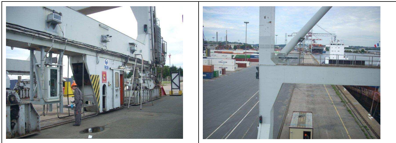
Figure 3: some of the boxes of the Cargo Monitoring Module prototype framing the container while moved
