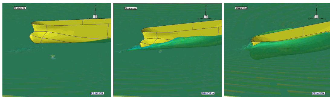
Fig. 2.4: 'Slamming of a ship bow'
