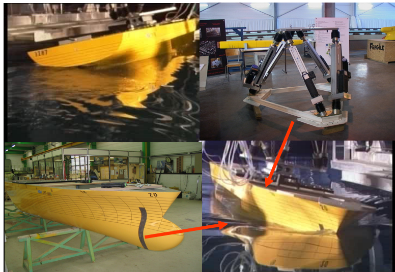
Fig. 2.1: 'Model test (HTC) for roll damping coefficients'
