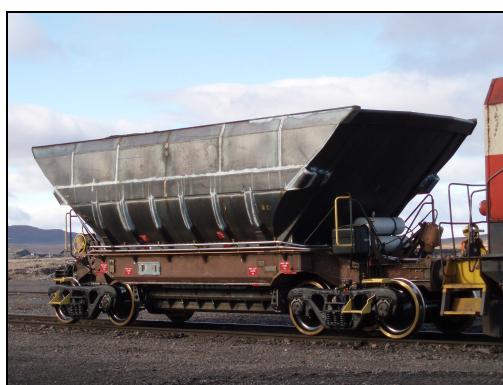
One of MTAB cars with 30 tonne axle load
