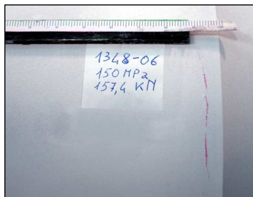
Example of fretting fatigue crack
