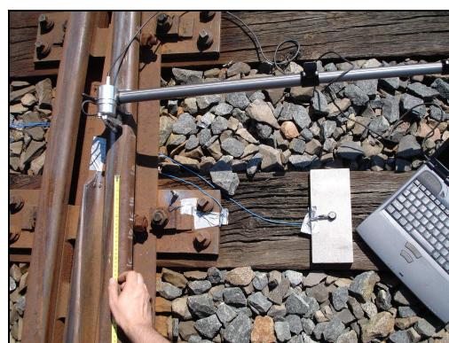
Switch profile measurements measurements during passage over switch
