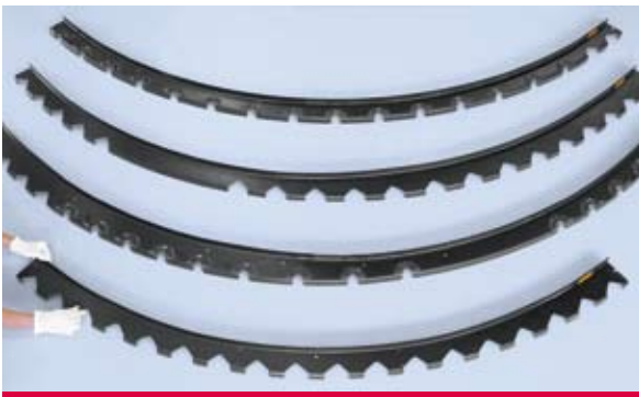
Fuselage frame sections in CFRP composite material (FP5 TANGO project)
