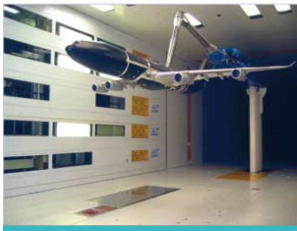
New Acoustic Phased Array Measurement Technique in DNW-LLF Wind Tunnel used in AWIATOR Technology Platform under FP5. (courtesy NLR)
