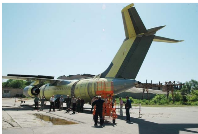
AN-148 – Sections made of composite material are grey coloured (Image courtesy of Antonov ASTC)
