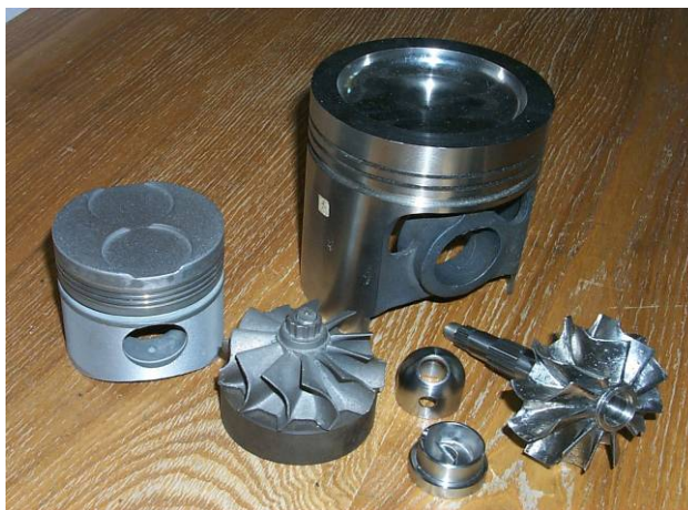
Transmission components made from novel titanium composites (tribotic) (Image courtesy of IPMS-NASU)
