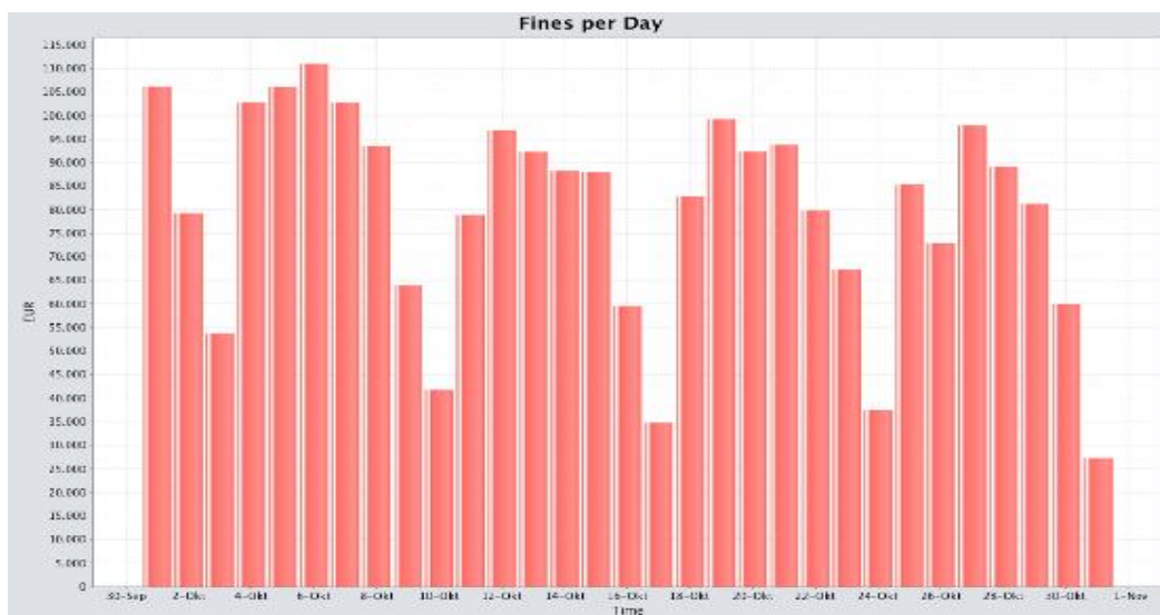
Figure 38: Example of possible fines per day based on overloaded trucks on a typical month (October 2010) computed from the weigh-in-motion system.
