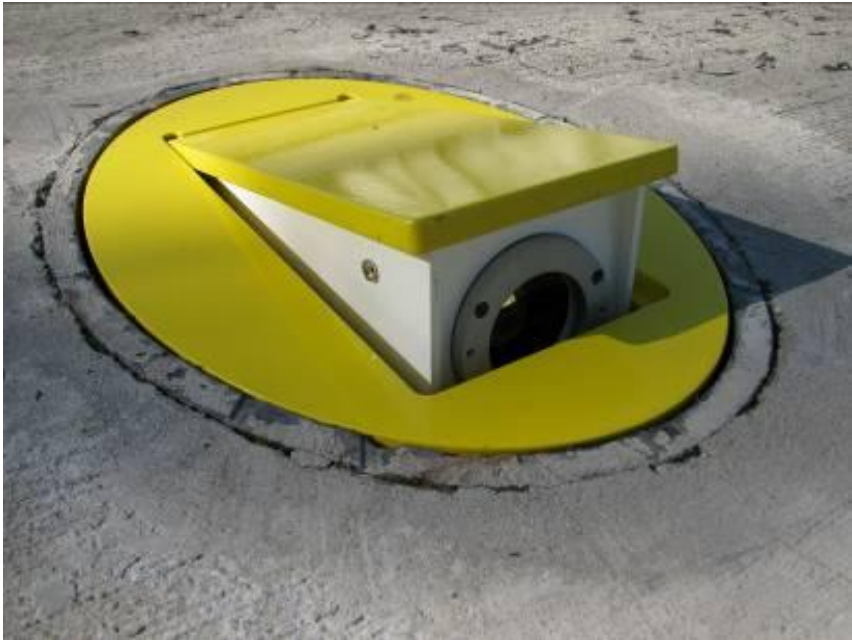
Figure 44: Thermal camera for observing all trucks regarding brakes, tires and power line conditions from below while they are passing the control station.
