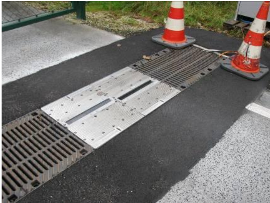
Figure 45: Tire profile measurement system for detecting too less profiles of all trucks passing the control station.
