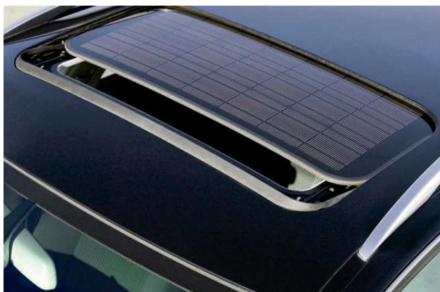
Figure 2-11 Solar cells integration 2008 (source: Webasto Solar)
