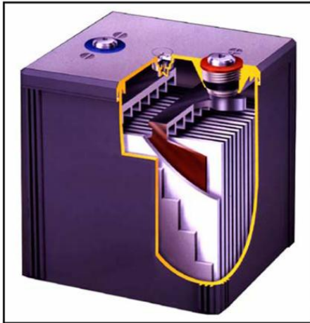
Figure 2-13 Internal structure of an AGM battery (source: wikipedia)
