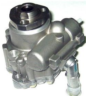
Figure 2-34 Illustration of a hydraulic steering pump
