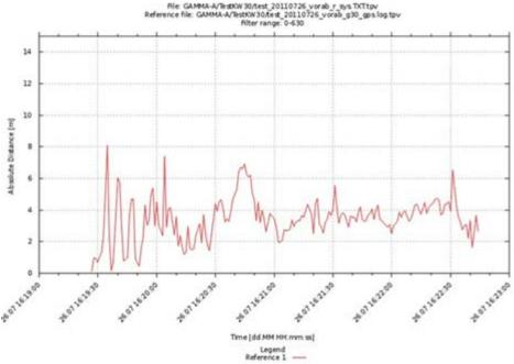
Differences in meter between GAMMA-A fusion solution and reference solution
