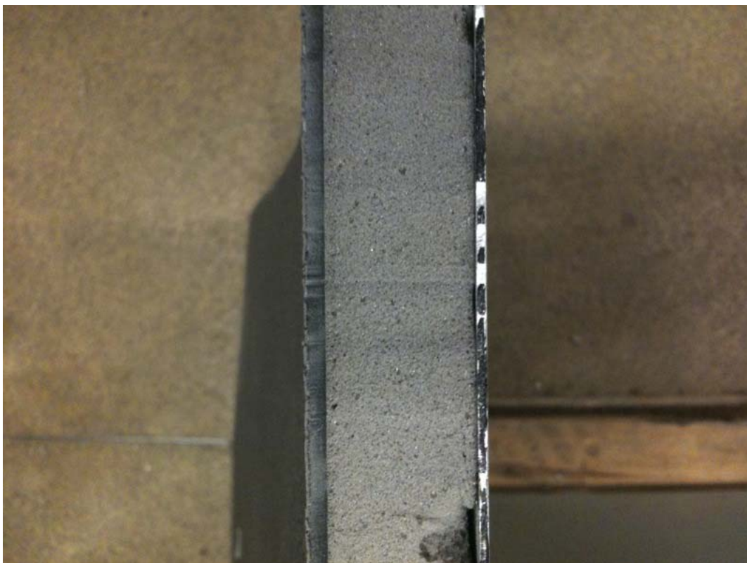
Figure 1 From left to right, the aluminium panel, Grey porous material and the rubber mat. The porous material is 2.24 cm thick.
