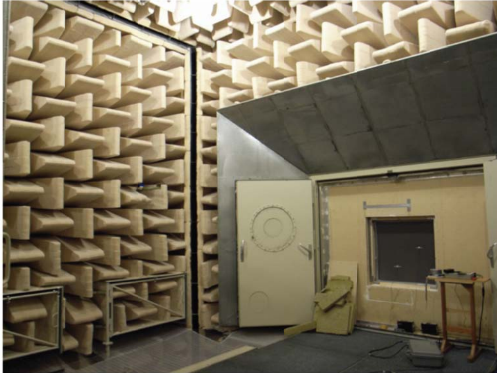
Figure 7 View of the multilayered structure from the anechoic room, where an intensity probe measures the time-averaged intensity.
