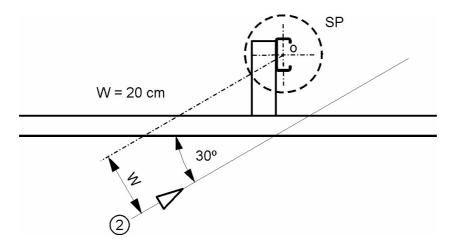
Fig. 3: Trajectory 2: Off-Centre Impact (Top View)
