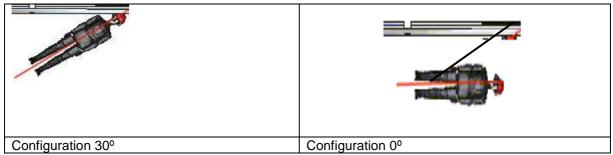
Figure 1: Impact configurations of the test proposed by LIER (France)
