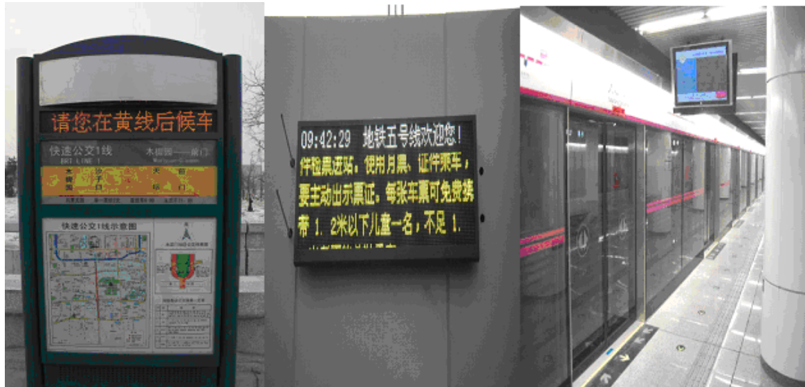
FIGURE 38 VARIABLE MESSAGE SIGNS
