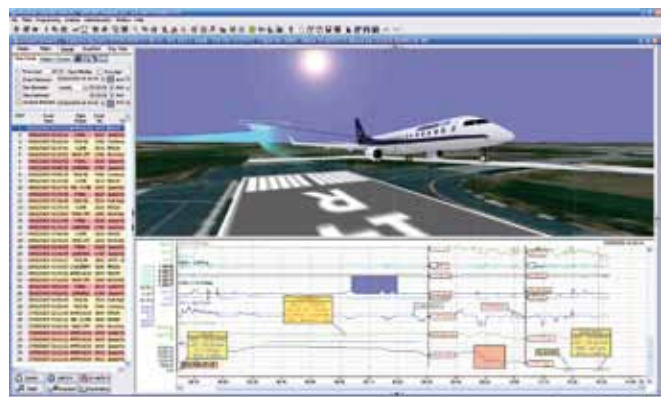
Use of AGS software to analyse flight data (charts and 3D) in the case of a landing following a go-around.
