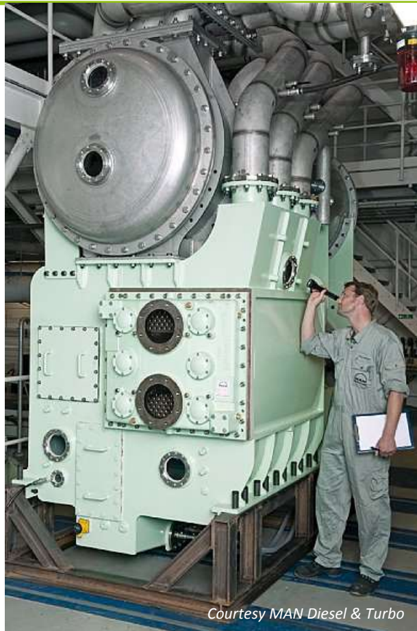
Figure 58: EGR system scrubber unit
