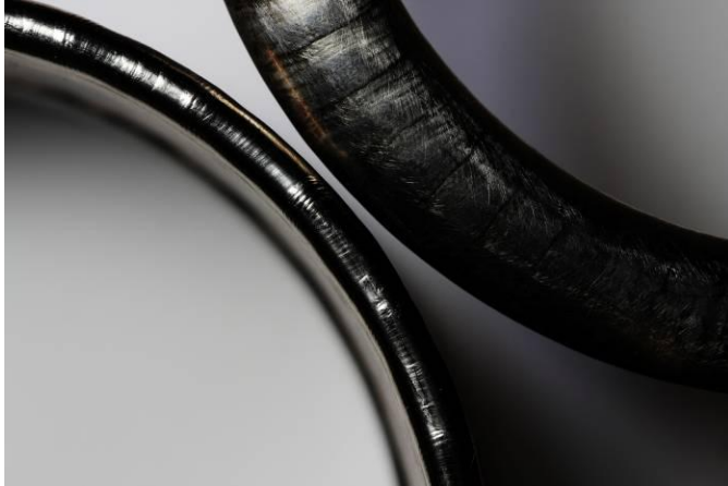
Figure 3: Different wall widths obtained after optimisation
