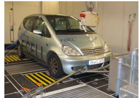
Figure 1: A-Class F-CELL in Vela Laboratory
