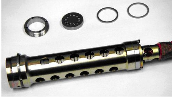
Fig.6.4.2 Piezo-actuator mounted inside of supporting tube of S/A ( I-23 )
