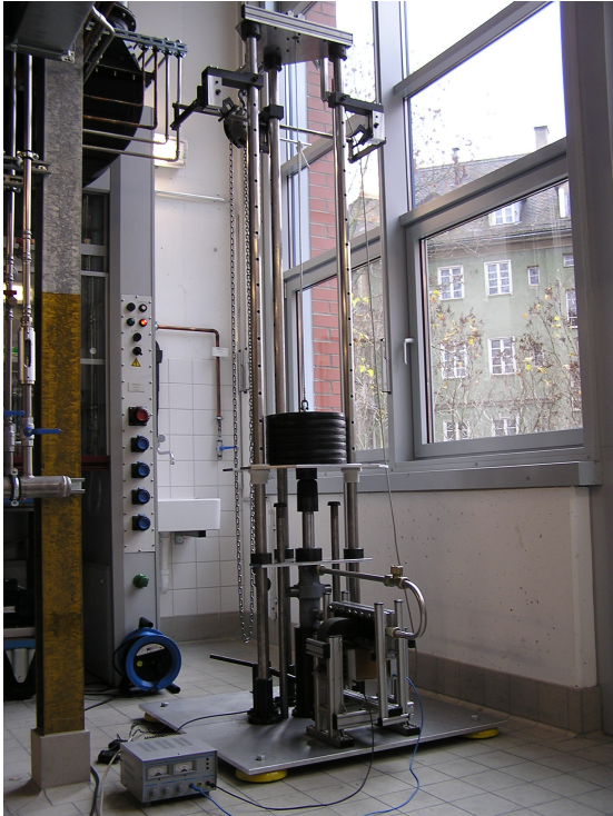
Fig. 6.5.5: Drop test device with shock absorber
