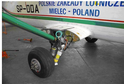
Fig. 6.4.6. Second prototype of SKYTRUCK's main L/G with adaptive shock absorber mounted to the structure of airplane.
