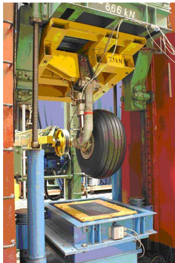
Fig. 6.4.5. New main L/G with adaptive shock absorber during drop tests in IA.
