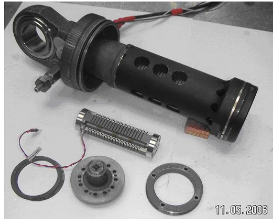
Fig. 6.4.4. Damping head with new piezo-actuator PPA80XL for SKYTRUCK
