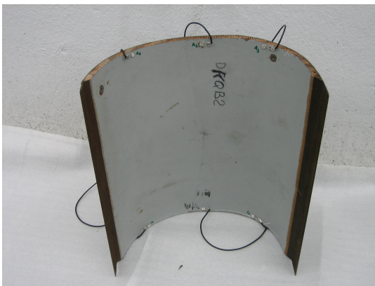
Fig. 21 Cut-out of EC135 tail boom
