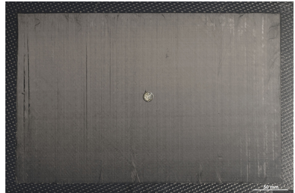
Dry fibre placement on generic preform and the injected preform
