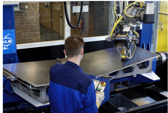
Example of AFP manufacturing. Thermoplastic tape placement of skin [ALCAS]
