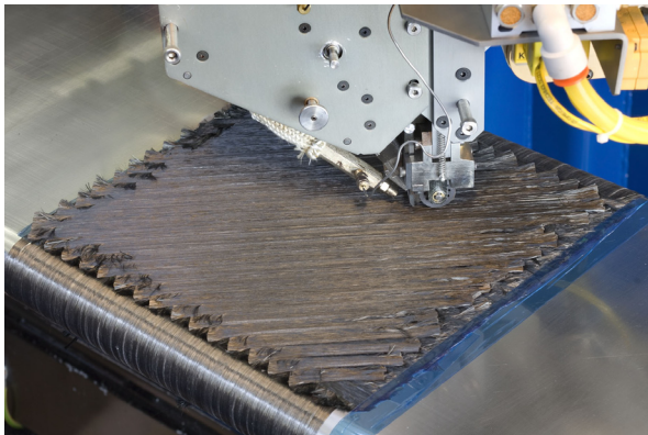
Dry fibre placement on generic preform and the injected preform
