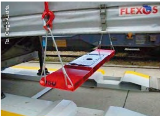
Figure 51: ISU equipment: cross beam under king pin
