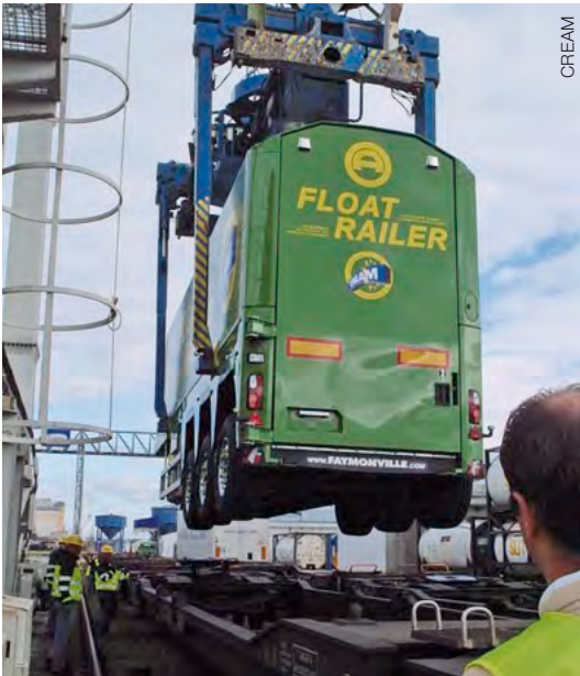
Figure 58: FLOATRAILER test loading by gantry crane (Worms, 12 Sep 2010)
