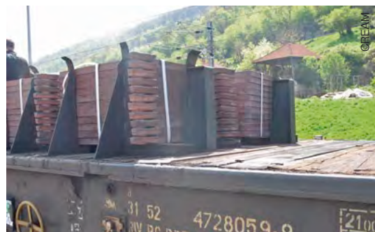
Figure 75: Transport of copper anodes on Smmps open flat waggons
