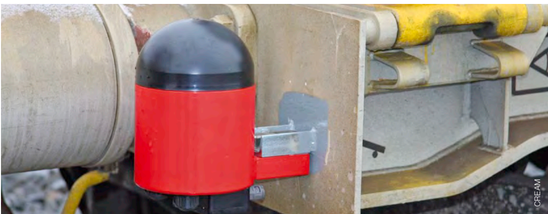
Figure 35: NavMaster GPS device for waggon tracking
