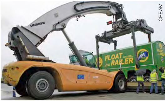
Figure 57: FLOATRAILER test loading by reach stacker (Genk, 8 Sep 2010)
