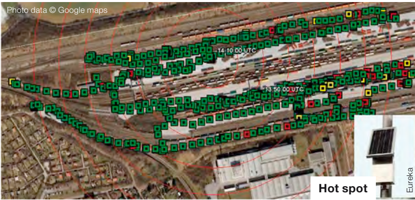
Figure 40: WPAN reading tests at a container terminal
