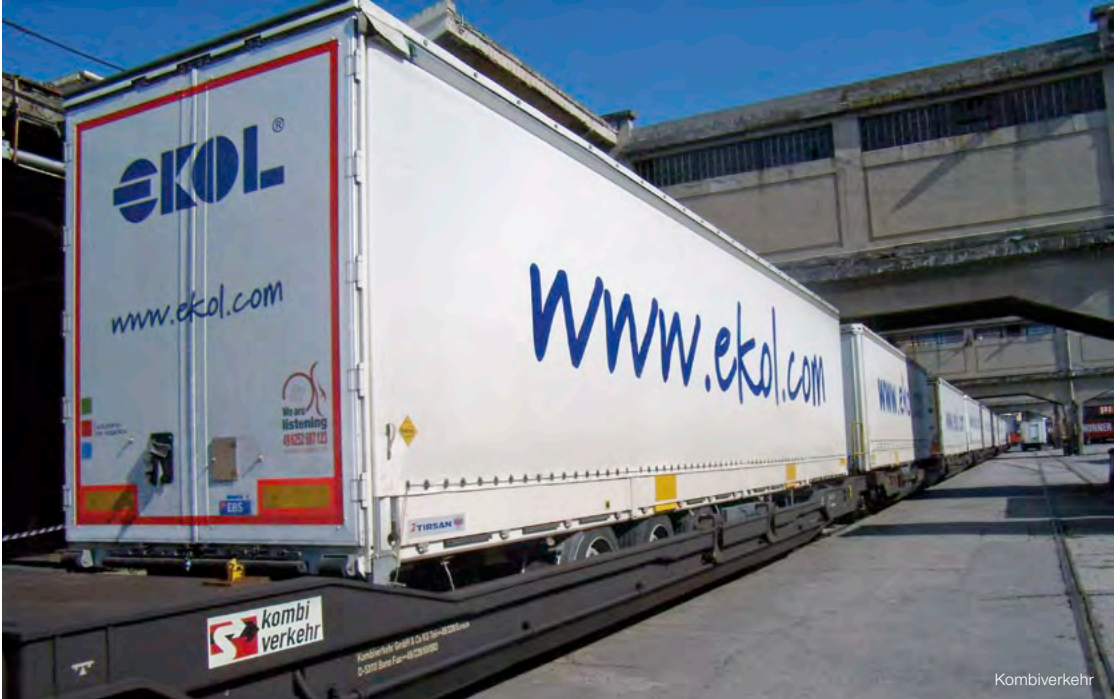
Figure 72: Ekol trailers loaded on Kombiverkehr pocket wagons (Trieste, October 2008)
