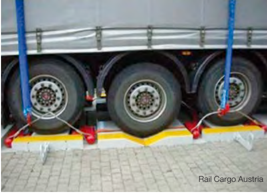
Figure 49: ISU equipment: wheel grippers
