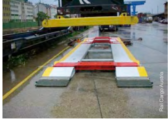
Figure 50: ISU equipment: loading platform prepared for truck/trailer
