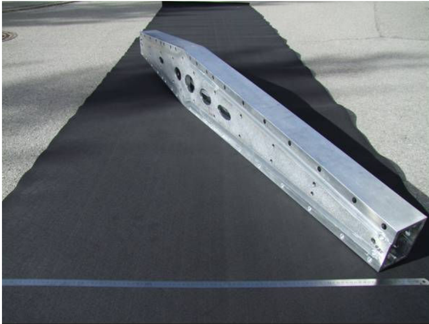
Figure 145: Total view of the DeltaN tool welded 2050 alloy beam track
