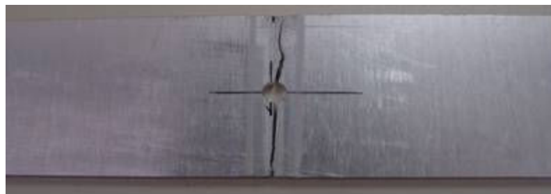
Figure 11: Test specimen after failure
