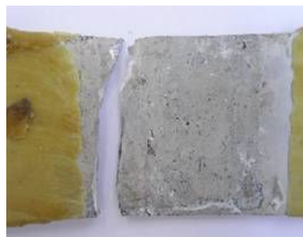
Fracture out of the heat affected zone (weld zone)
