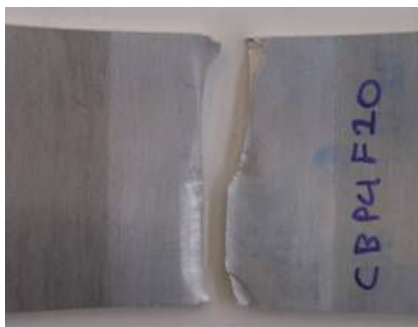
Fracture in the weld joint line
