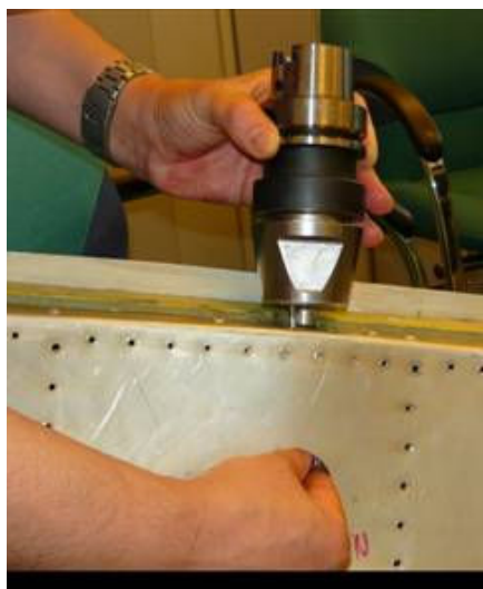
Figure 171: An economical and rapid repair in service requires the Pax Door isn't disassembled so Pai and Eads-G decided to use Bobbin Tool
