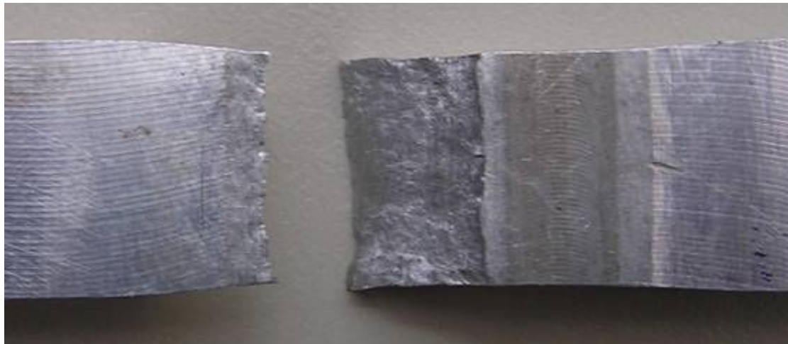
Figure 72: Bottom view of fractured specimen
