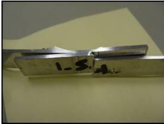
Figure 88: Examples of FSW lap joint in Al 2024-Al 7475 after fatigue testing by Piaggio
