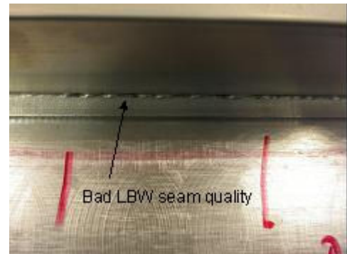
Figure 197: Example of large deformation caused from Laser welding of a stringer. In addition, in this particular case, the presence of gap between stringer and panel has led to a bad quality of LBW
