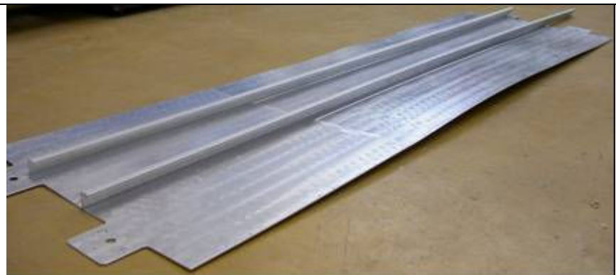
Figure 198: Friction Stir Welding of concept 4 having LBW stringers (V534-H1504-006)
