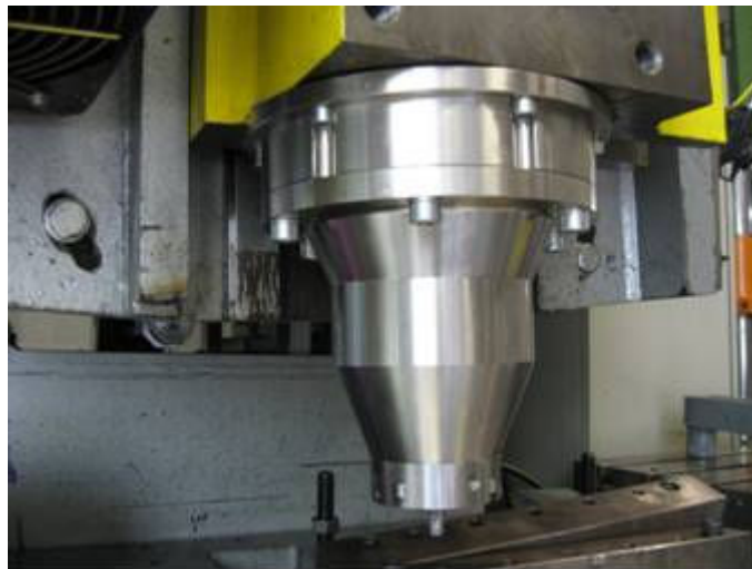
Figure 241: DeltaN tool generation 4 tool case fixed at the lower end of the ESAB Superstir welding head
