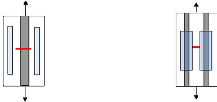
Figure 7: Positions of retarder straps in 2198 single (left) and double weld (right) configurations.
