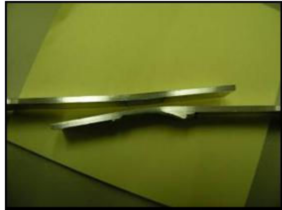
Figure 88: Examples of FSW lap joint in Al 2024-Al 7475 after fatigue testing by Piaggio
