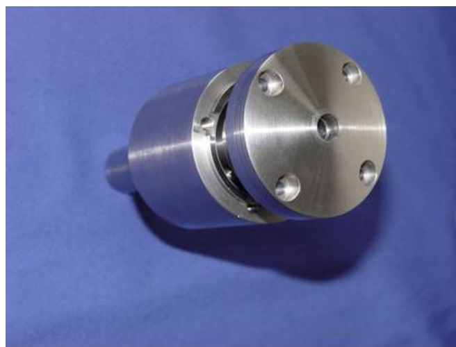
Figure 240: Top view of DeltaN tool generation 3 shoulder cup and tool case
