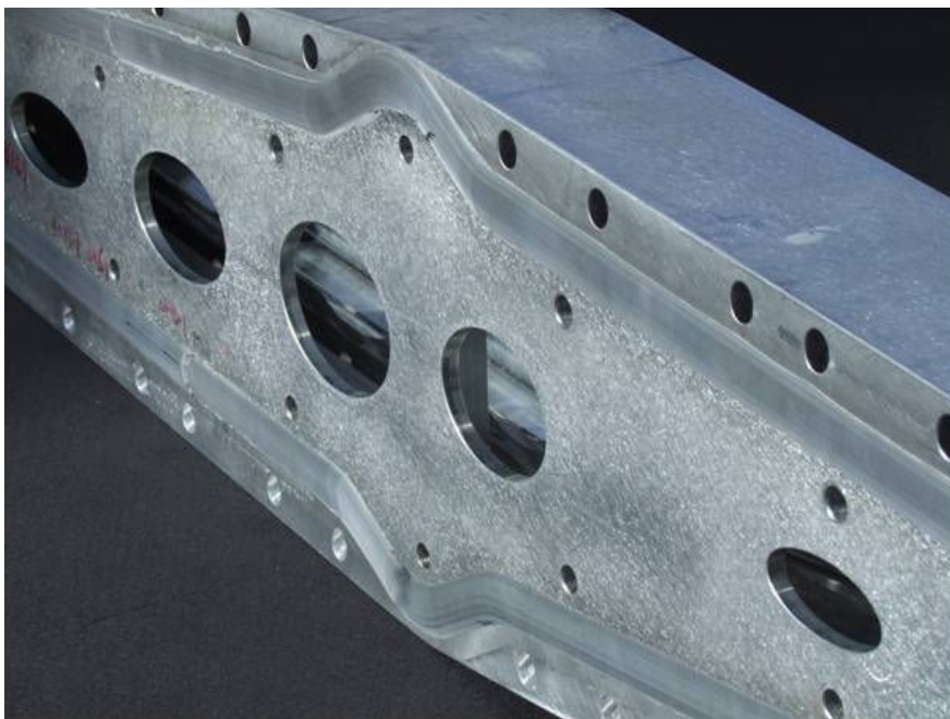
Figure 146: Detail view of the DeltaN tool weld top surface and its superb surface finish
