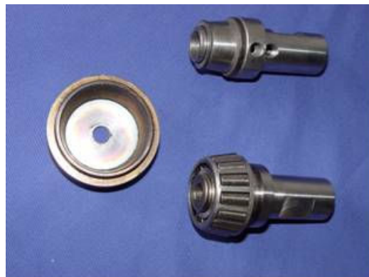
Figure 236: Shoulder cup, shaft and bearing as the three main components of the DeltaN tool concept
