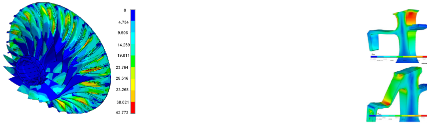
Figure 50: Relative impeller vibration stresses; Distribution of relative equivalent stresses in free turbine stage
