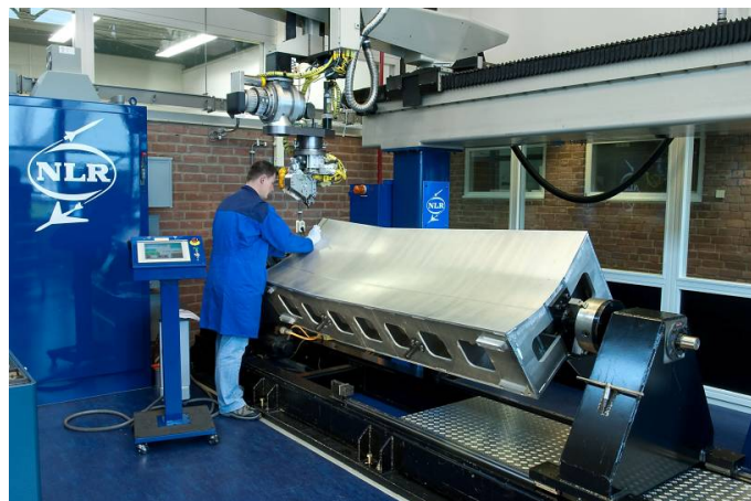
Figure 21: Fiber placement machine with skin mould
