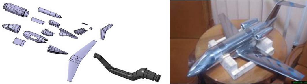
Figure 6: Wind tunnel model of AC2 with optimized turbulent wing
