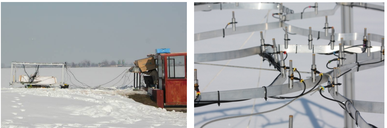
Figure 65: Test set up for noise mapping measurements through beam-forming technique
