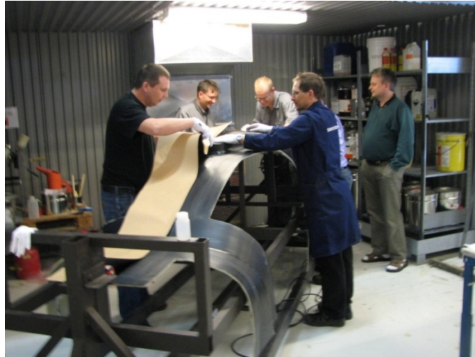
Figure 24: Lay-up of the roof
