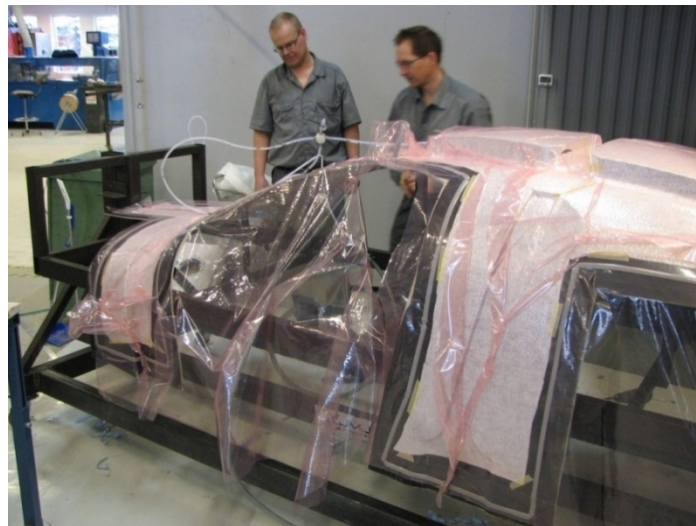
Figure 25: Set-up of the roof for the out-of-autoclave cure at SICOMP
