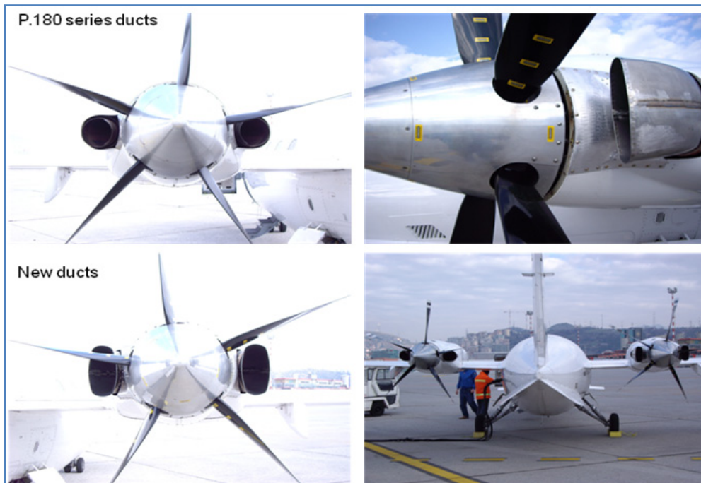
Figure 64: Manufacturing and installation of new gas exhaust ducts on P.180 experimental aircraft
