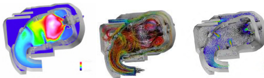
Figure 51: Combustion Chamber CFD simulation results (FOI)
