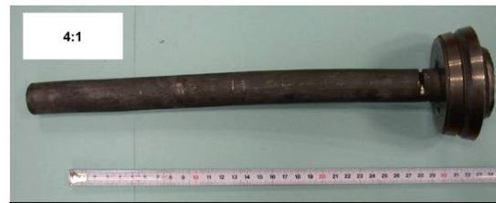
Fig. 8. Extruded Nb-silicide alloy based on MASC composition (PM route).
