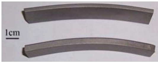
Fig. 7. Investment cast Nb-25Ti-8Hf-2Cr-2Al-16Si generic engine seal segments with different thickness.
