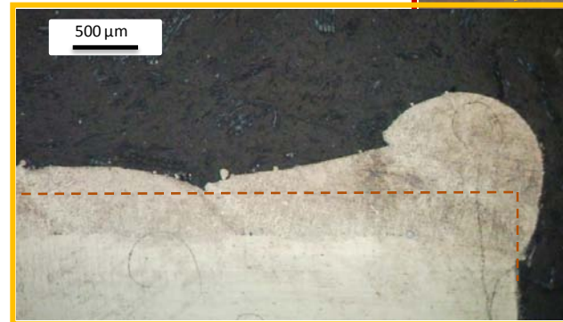
LMD around holes. Blue broken line depicts section required after machining
