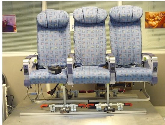
Figure 44: Vibration control platform
