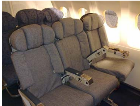
Figure 38: Thales Mock-Up : Integrated SEAT in Cabin Environment
