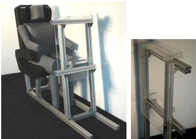
Fig. 10 Left - laboratory set-up of single seat personalized ventilation system, right – detail of the pair of nozzles built in the laboratory seat set-up.
