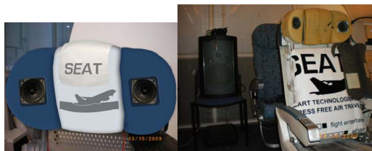
Figure 42: Integration of speakers into the seats.
