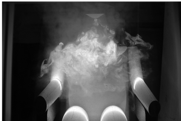
Figure 12: Airflow distribution in the seat area visualized by SAFEX fog
