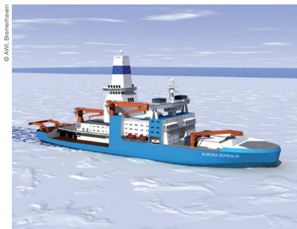
Figure 11. The Aurora Borealis icebreaker was endorsed by the European Polar Board in early 2000. The vessel provides unique capacities to carry out interdisciplinary research in almost 90% of polar waters in any season and weather conditions. The model underwent severe tests for both frontal and lateral ice-breaking capabilities in Hamburg and in Finland at the Aker Arktic's towing tank.
