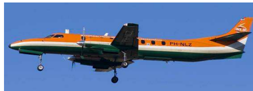
NLR's Swearingen Metro II aircraft, a twin turboprop aircraft, modified for aerospace research. (Image provided by NLR.)
