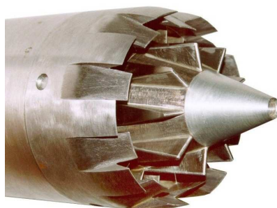
Figure 68 – Proposed plug sector nozzle to reduce noise
