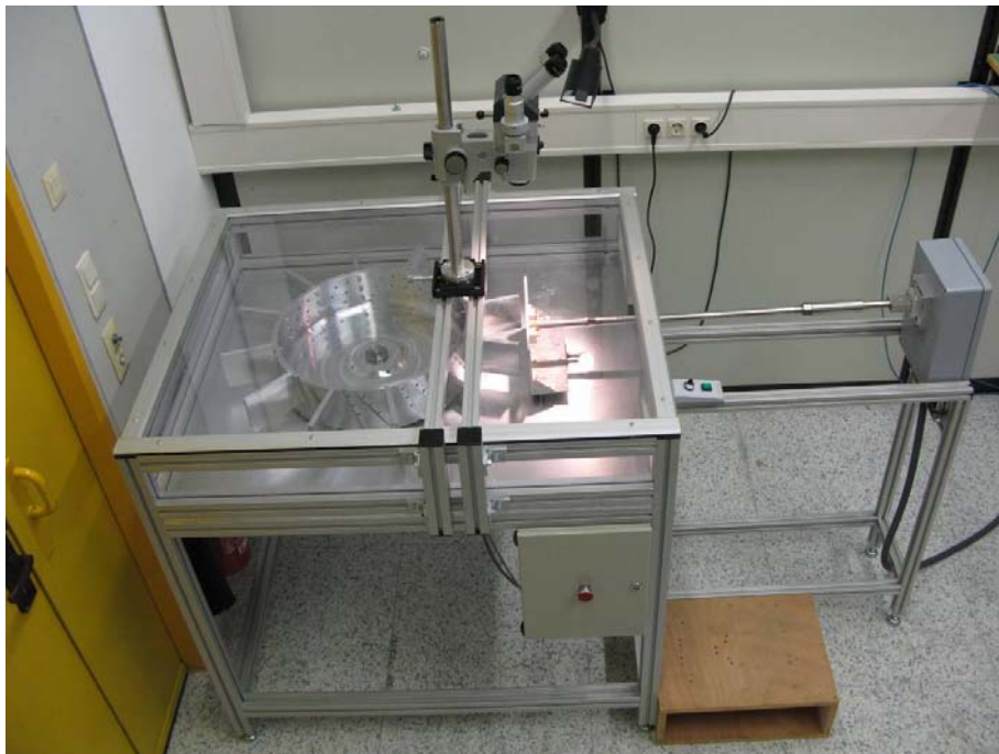
Figure 47: Rotating rig with mm-wave probe
