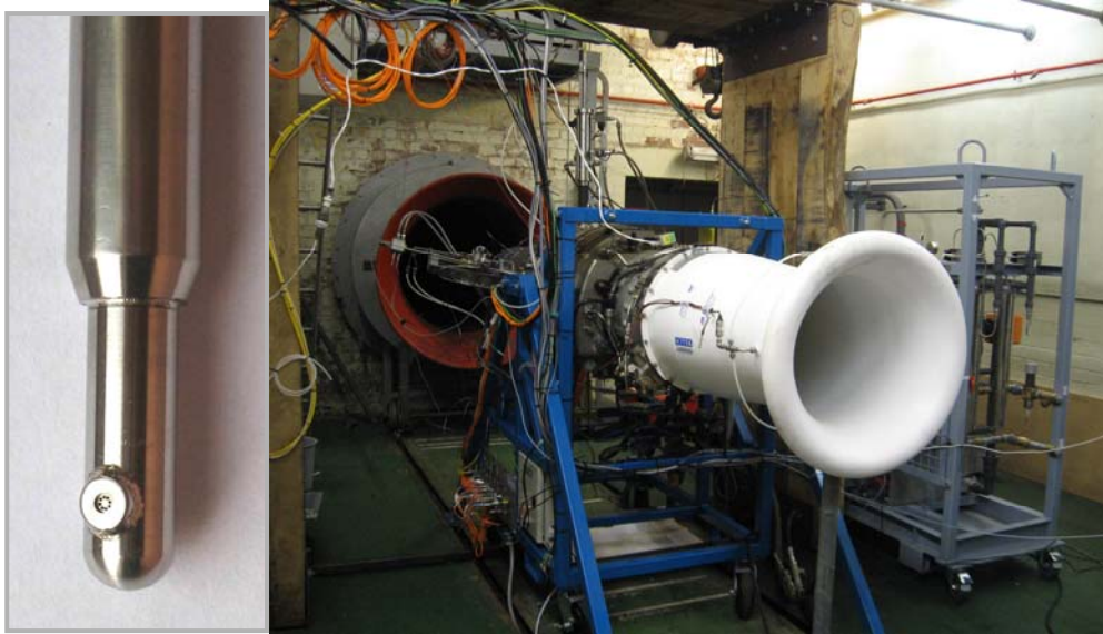
Figure 24 Fast response cooled total pressure probe (left) and first engine measurements in a Rolls-Royce Viper gas turbine exhaust (right)
