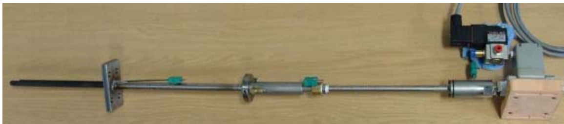
(1) (2) (3) (4) Figure 29: Picture of a probe prototype: (1) probe head, (2) cooling system, (3) mass flow meter, (4) on/off valve. Downstream the system – not depicted in the picture is the gas analyser.
