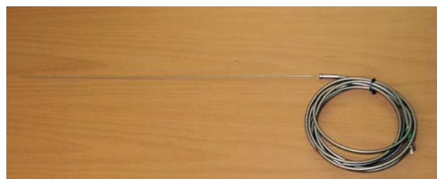
Figure 13: High Temperature FBG sensor. 3 measurement points are sequentially arranged in the probe.
