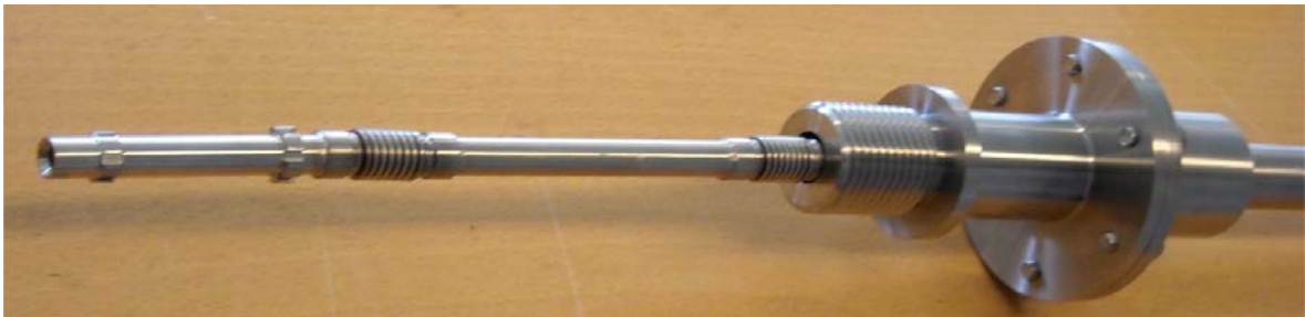
Figure 17: KEMA borescope pyrometer with refractive optics
