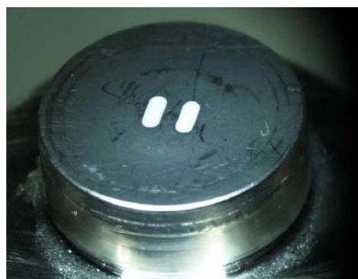
Figure 44: Sensor tip with sealed antenna
