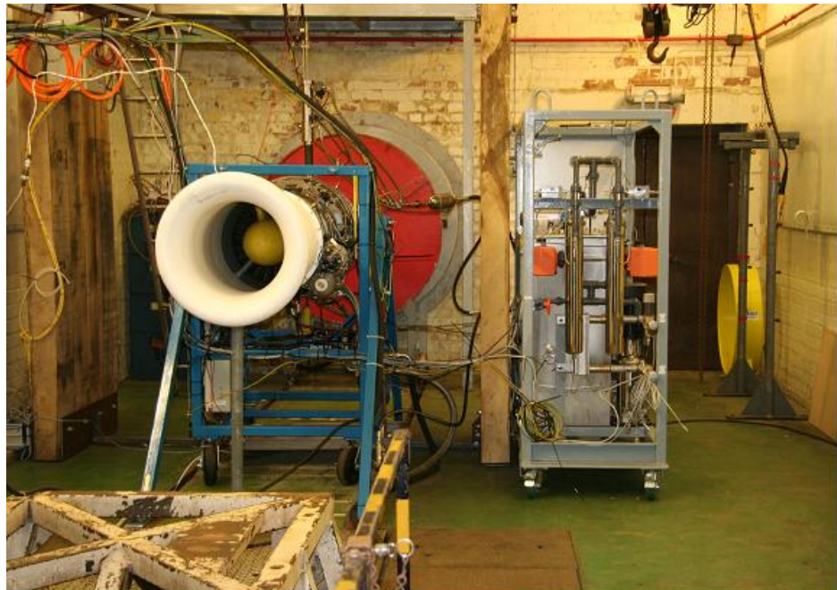
Figure 49: Viper 201 engine on 42 test bed at Rolls-Royce Ansty (VKI probe cooling system installed to left of engine)
