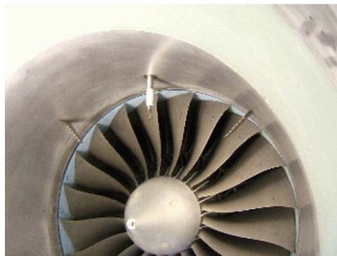
(c) Inlet flow hot-wire probe
