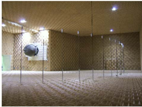
(a) Fan rig installed in anechoic chamber
