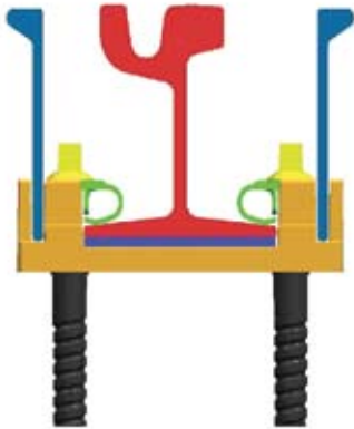
Figure 1: assembled view of the developed track system, to be poured in concrete (on site) or mounted in pre-cast concrete slabs
