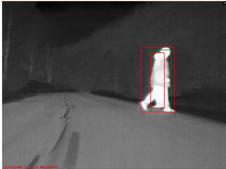
Figure 21. An image in which the system output is highly similar to the ground truth but misses a salient pedestrian.
