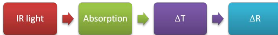
Figure 20. The multi-step process of converting IR radiation to a resistance change that can be measured and interpreted as an image.
