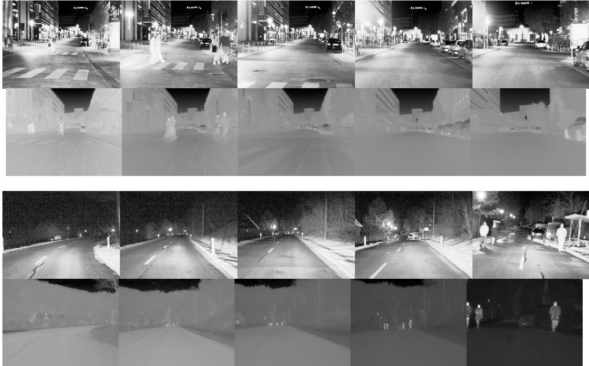
Figure 8. Two examples of FIR (top) and NIR (bottom) images from the measurement campaign that used five different optics configurations in hot weather.
