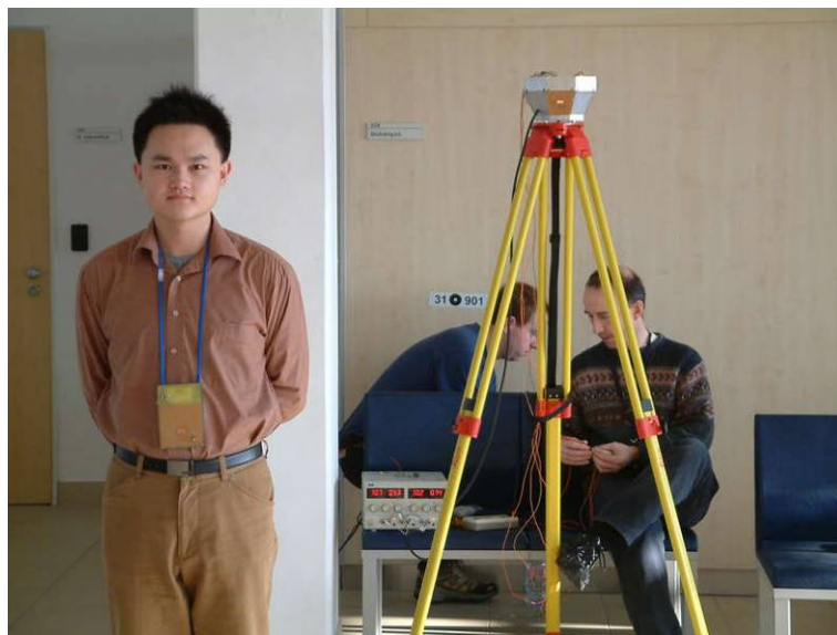
Manually measuring the RF signal received from a tag facing away from the reader
