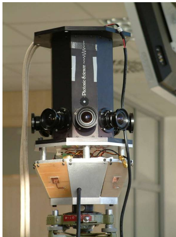
A close-up of an OpTag camera cluster (top) and RFID reader module (bottom)
