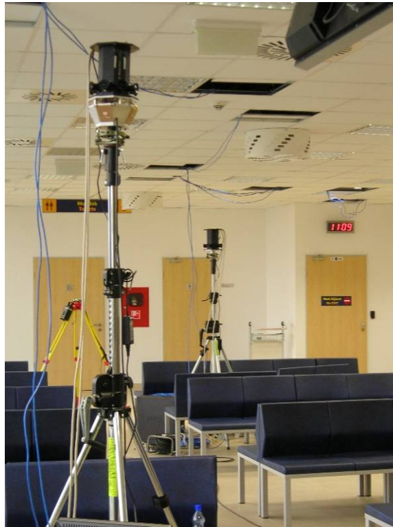
Debrecen Airport departure lounge showing two OpTag readers mounted on tripods
